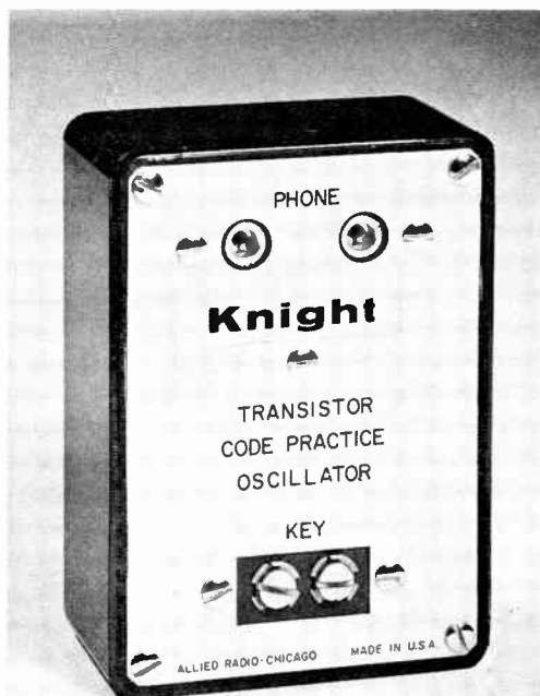
THE KNIGHT CODE PRACTICE OSCILLATOR This oscillator is a simple tickler coil audio oscillator similar to Fig. 3.8-A. (Photo by Allied Radio)
