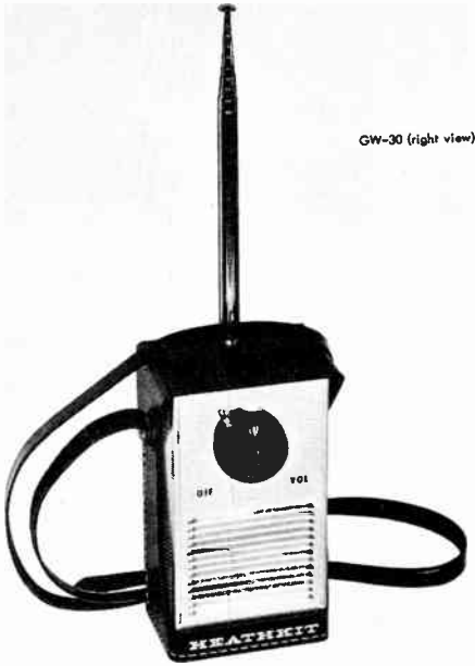
THE HEATH GW-30 May be easily converted to 10-meter operation by replacing the crystal and retuning the receiver and transmitter coils. (Courtesy of Heath)
