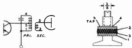
Figure 4.8-C Construction details for the home-made 455 kc. transistor i.f. transformers.
