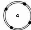
Figure 1.3-C A SIMPLIFIED DRAWING SHOWING ONLY THE VALENCE ELECTRONS This could be either the germanium or silicon atom since they both have four valence electrons.
