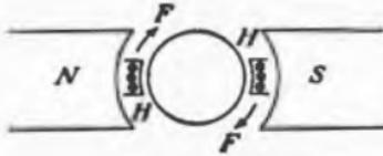
FIG. 1.—Moving-coil galvanometer.
