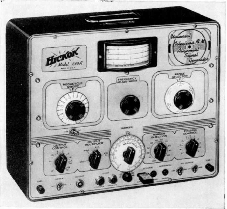
FIG. 19-16. TV sweep generator for alignment. R-F range 30 to 230 Mc; output up to 0.5 volt; 4.5 Mc crystal for intercarrier-sound i-f alignment; sweep width 15 Mc or 1.5 Mc; sweep rate 60 cps; marker absorption dip or oscillating pip frequency range 19 to 48 Mc. (Hickok Electrical Instrument Company.)
