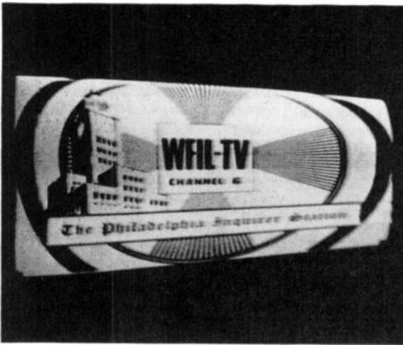
FIG. 18-41. Trapezoidal raster caused by defective deflection yoke. Keystoneing at top and bottom shown here produced by shorted vertical coil. Keystoneing at sides can be caused by shorted horizontal coil. (RCA.)
