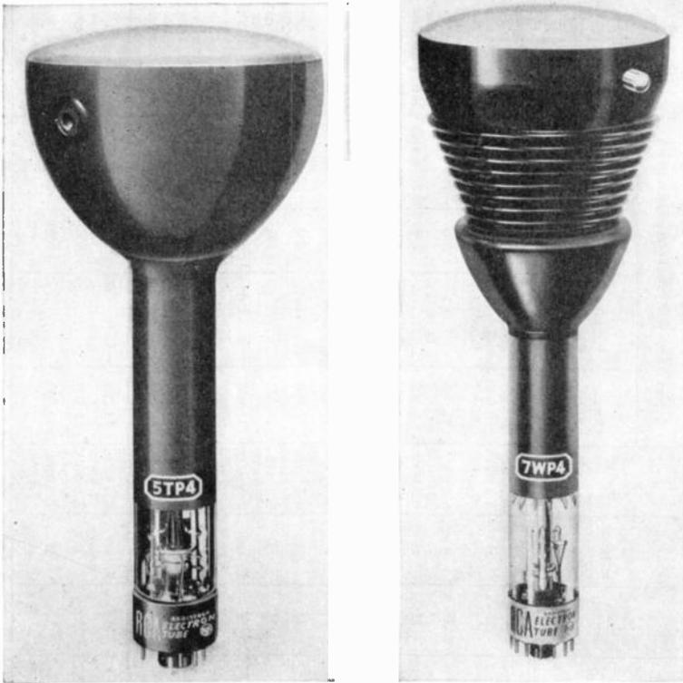
FIG. 9-8. Projection kinescopes 5TP4 and 7WP4. (RCA.)
