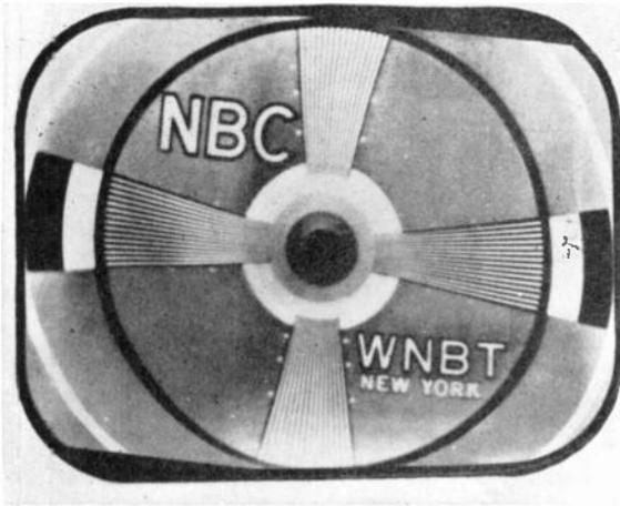
Fig. 23-3. Raster tilted with respect to mask because deflection yoke is tilted. (RCA.)
