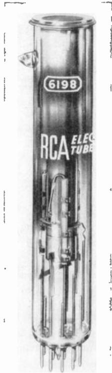
FIG. 2-13. The vidicon camera tube. It is  $6\frac{1}{4}$  in. long and 1 in. wide, approximately. (RCA.)
