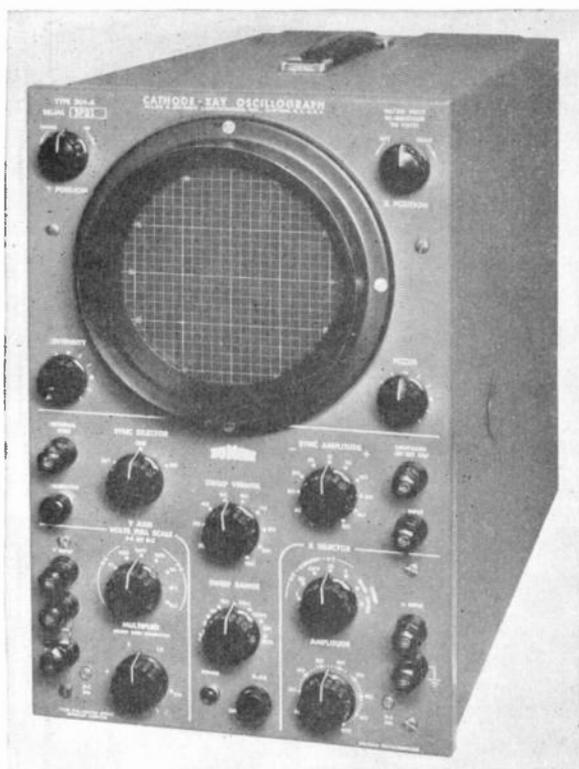
FIG. 23-10. Typical 5-in. oscilloscope. Frequency response of vertical amplifiers is from d-c to 100 ke within 1 db. Internal-sweep frequency range 2 to 30,000 cps. (Allen B. DuMont Laboratories, Inc.)
