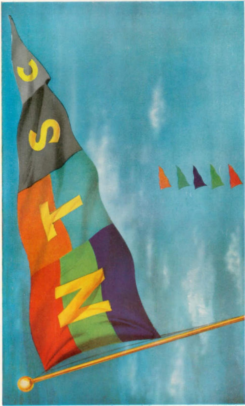
PLATE VII. NTSC flag illustrating color resolution in color television. Largest areas in full color as mixtures of red, green, and blue; smaller areas in cyan and orange; smallest details in black-and-white. (From *Proceedings of the IRE, Second Color Television Issue, Jan. 1954.*)
