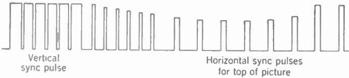
FIG. 16-27. Weak horizontal sync following the vertical pulse. Not drawn to scale, as reduced amplitude of horizontal pulses can continue for many more scanning lines at the top of the picture.
