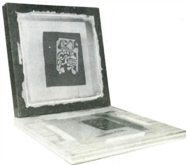
Figure 8-2D: Silk screen jig for producing printed circuit patterns
