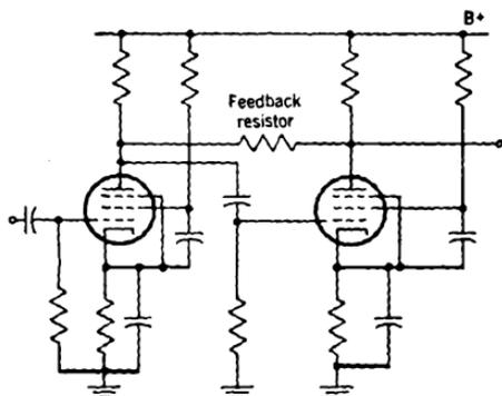
FIG. 2-21.—Feedback from plate to preceding plate.
