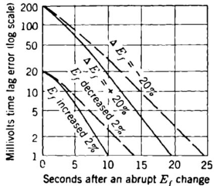
FIG. 11-8.—Heater-cathode time lag of a 6SL7.
