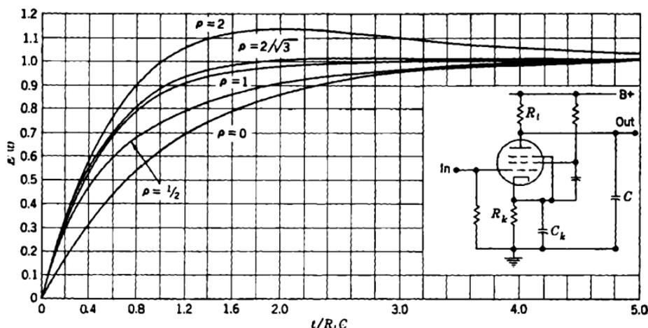
FIG. 2.20.—Step-function response of cathode-peaked pulse-amplifier stage,
