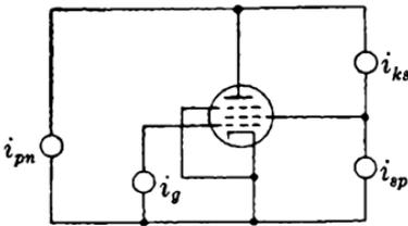
FIG. 13-3.—Equivalent noise representation for a pentode.
