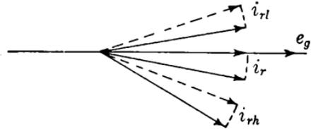
FIG. 6-14.—Correction of transit-time effect off resonance.
