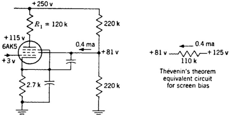
FIG. 9-19.—Preliminary design of pentode stage.
