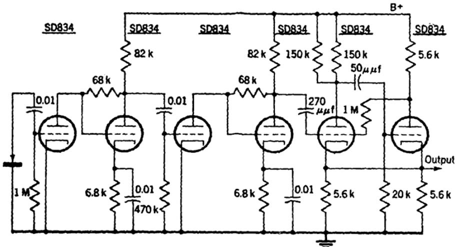
FIG. 3-39.—Circuit diagram of amplifier No. 2.
