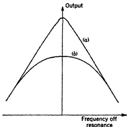
FIG. 6-1.—Amplifier response, (a) without feedback, (b) with inverse feedback.
