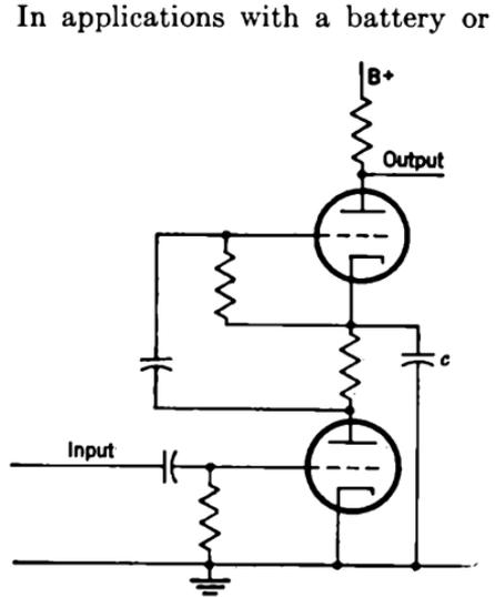
FIG. 3-33.—Series-fed circuit.
