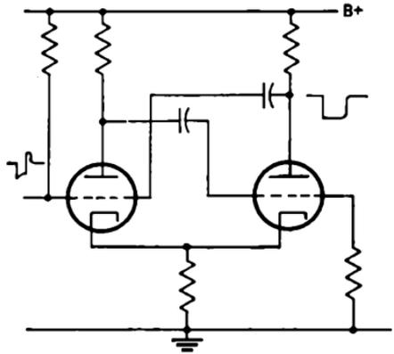
FIG. 3-27.—Multivibrator output stage.
