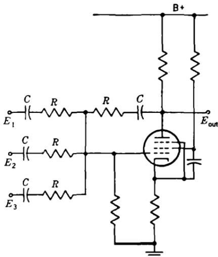
FIG. 2-31.—Typical three-channel feedback-amplifier mixer.
