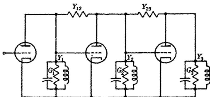
FIG. 6-5.—Feedback triple using single-tuned circuits.
