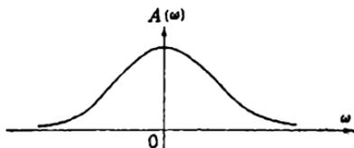
FIG. A-1.—Gaussian-error-curve filter,
