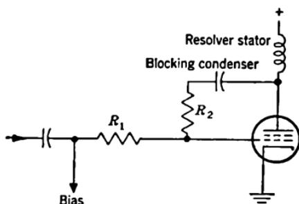
FIG. 9-11.—Single-stage driver with plate-to-grid feedback.
