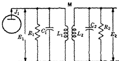
FIG. 5-1a.—Inductance-coupled double-tuned circuit.
