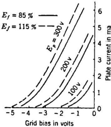
FIG. 11-7.—Effect of heater voltage on 6SL7 characteristics.
