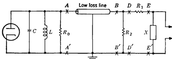
FIG. 14-5.—Matched-line diode noise generator.
