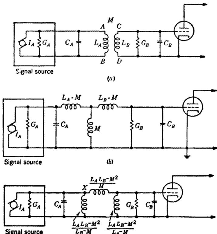
FIG. 13-25.—Double-tuned inductively coupled input network; (a) mutual-inductance-coupled circuit, (b) self-inductance-coupled T-circuit, (c) self-inductance-coupled  $\pi$  circuit.
