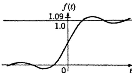
FIG. A-4.—Step-function response of idealized low-pass filter.
