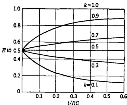
FIG. 2-24.—Step-function response for partially compensated potentiometer.
