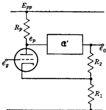
FIG. 11-53.—Over-all cathode feedback.
