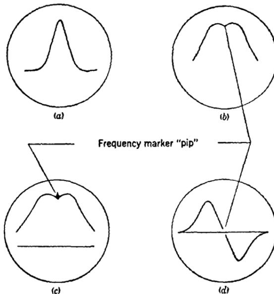
FIG. 8-2.—Typical response curves observed with a swept-frequency signal generator.
