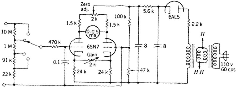
FIG. 11-62.—Simple vacuum-tube voltmeter.
