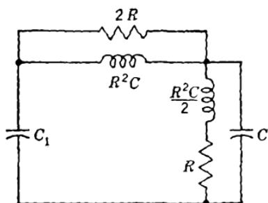
FIG. 2-10.—Series shunt-peaked circuit.
