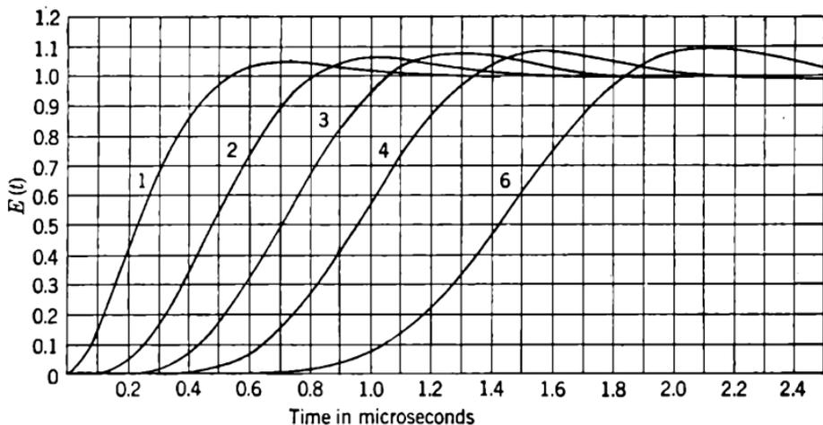
FIG. 7-5.—Step-function response of cascade of  $n$  flat-staggered pairs,  $n = 1, 2, 3, 4, 6$ , each pair of bandwidth 2 Mc/sec between 3-db points. These curves also apply to transitionally coupled double-tuned circuits, flat inverse-feedback pairs, and in general to all minimum-phase circuits having absolute value vs. frequency curves of the form  $1/\sqrt{1+z^2}$ .
