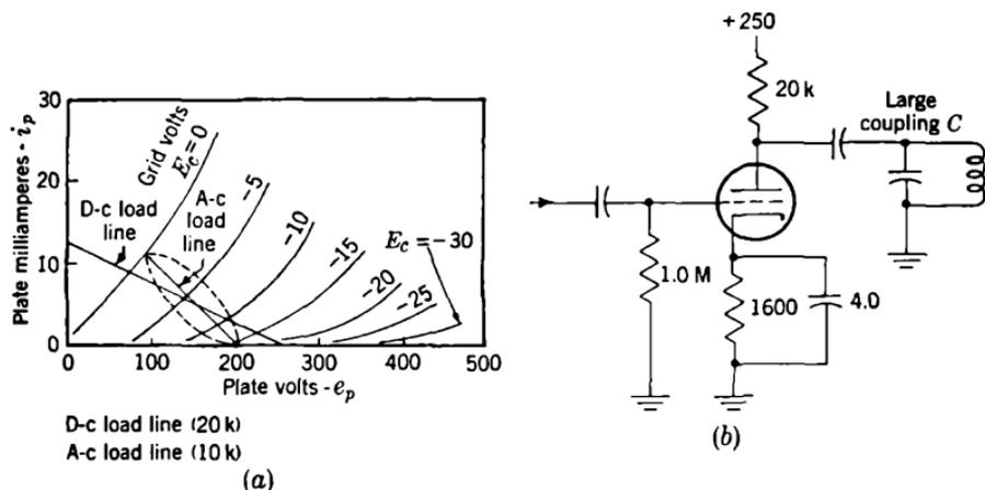
FIG. 9-15.—Operation of 6C4 output stage.
