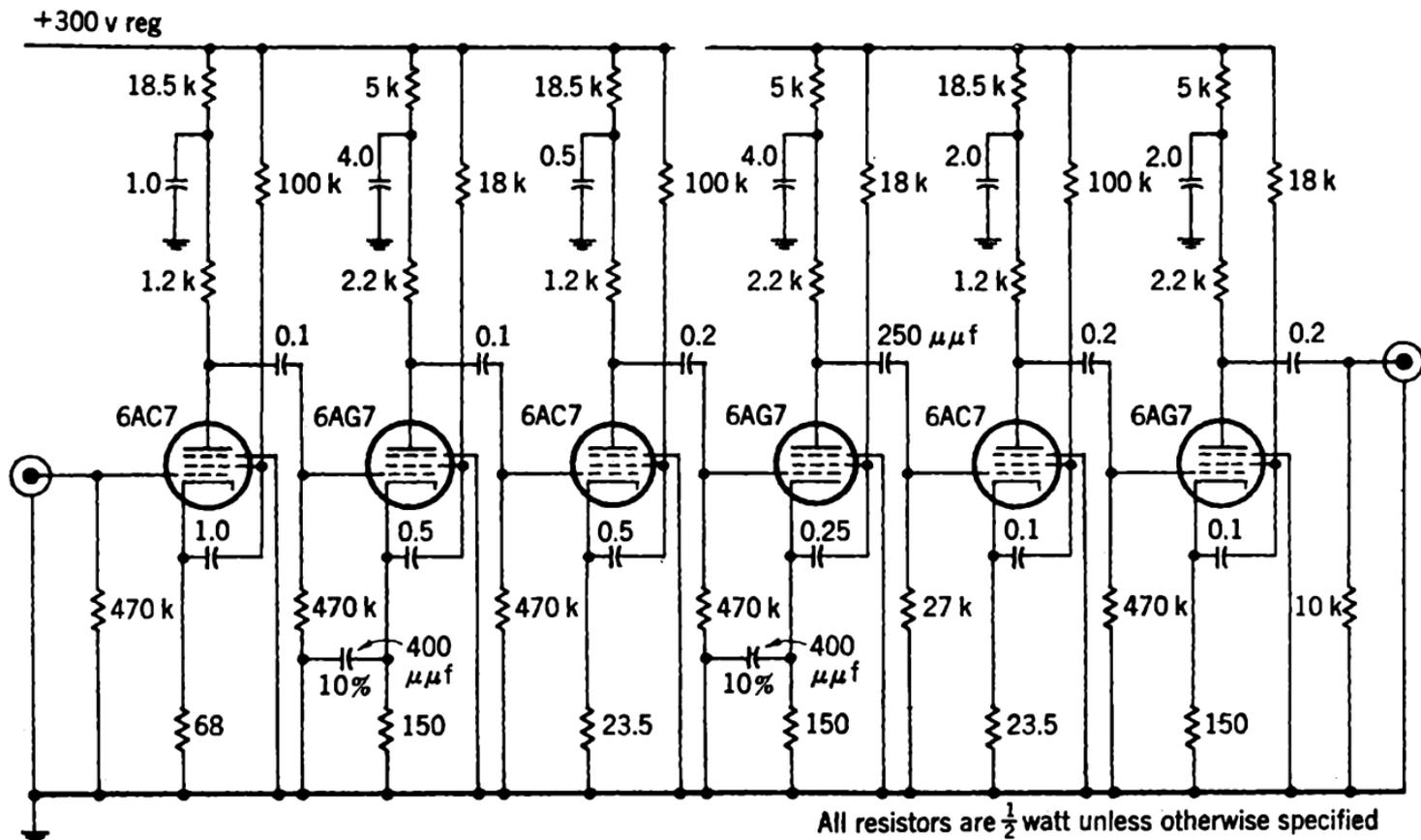
FIG. 3-36.—Complete circuit diagram for amplifier No. 1.
