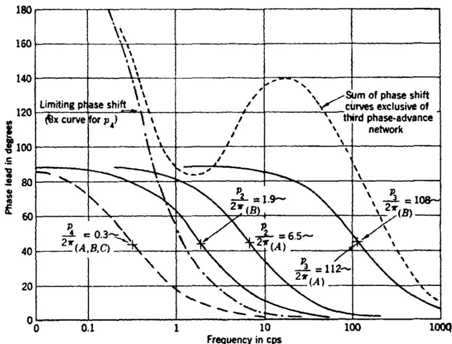
FIG. 9-31.—Phase characteristics for two stabilization networks.
