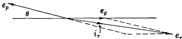
FIG. 6-11.—Vector diagram at resonance showing transit-time effect.
