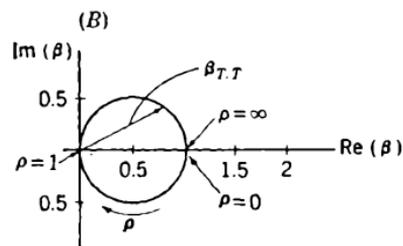
FIG. 10-2.—Phase-amplitude diagram of twin-T network.
