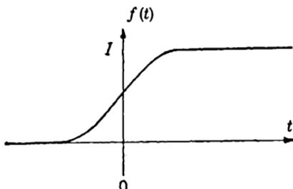
FIG. A-2.—Step-function response of Gaussian-error-curve filter.
