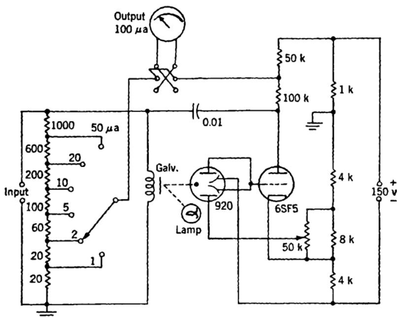
FIG. 11-72.—Microammeter based on Fig. 11-71c.
