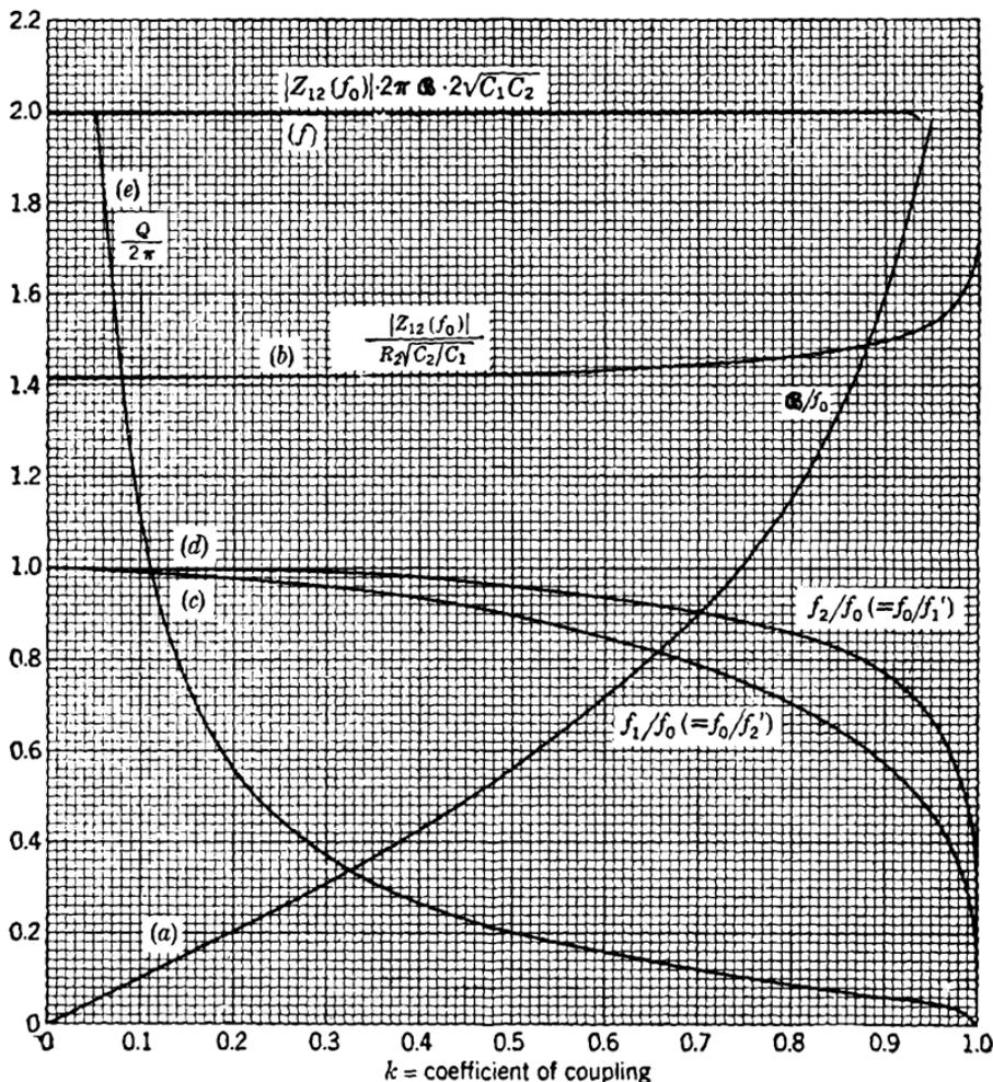
FIG. 5-7.—Design data for low- $Q$  transitionally coupled double-tuned circuit  $Q_1 = \infty$ ,  $Q_2 = Q$ . (a) Fractional bandwidth  $\mathcal{B}/f_0$ ; (b) normalized midband gain; (c) primary resonant frequency; (d) secondary resonant frequency; (e)  $Q/2\pi = f_0 R_2 C_2$ ; (f) gain-bandwidth factor  $|Z_{12}(f_0)| 2\pi \mathcal{B} 2\sqrt{C_1 C_2}$ .
