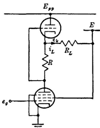
FIG. 11-39.—Series amplifier using pentode.
