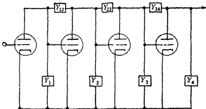
FIG. 6-3a.—Feedback chain using two-terminal shunt impedances.
