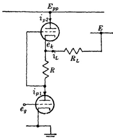
FIG. 11-38.—Series amplifier with load.
