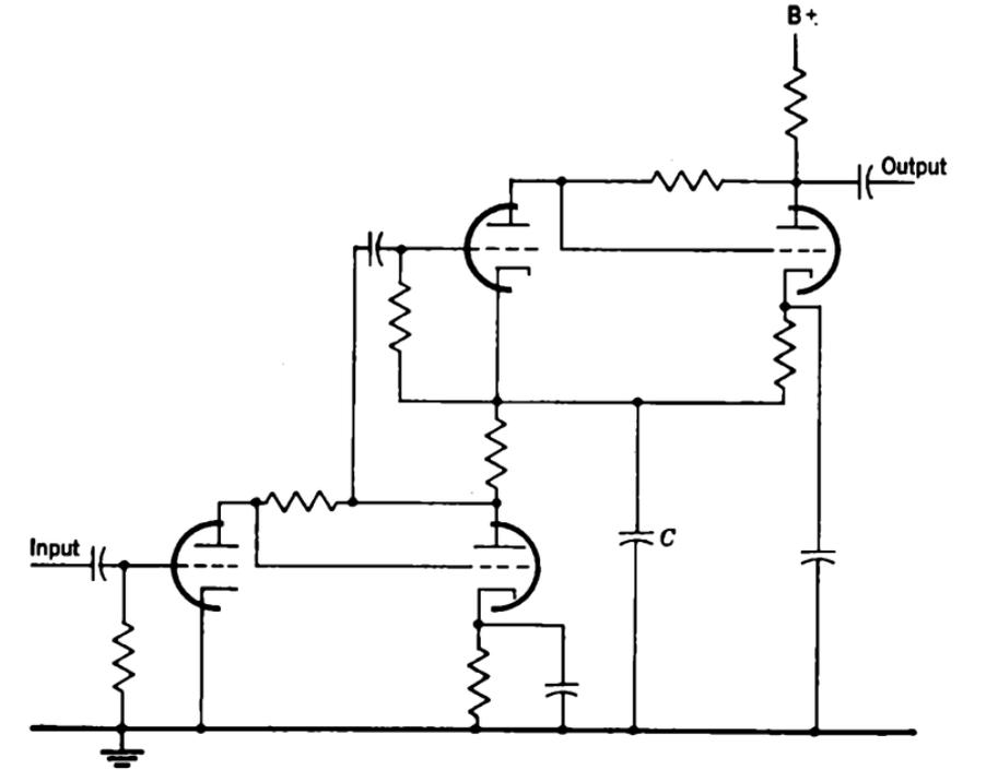
FIG. 3-34.—Series-fed direct-coupled inverse-feedback pairs.
