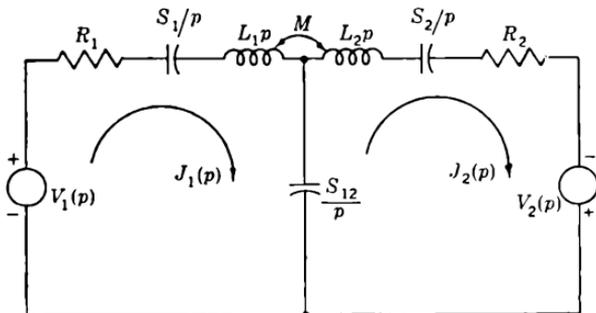
FIG. 1·19.—Two-mesh transform network.
