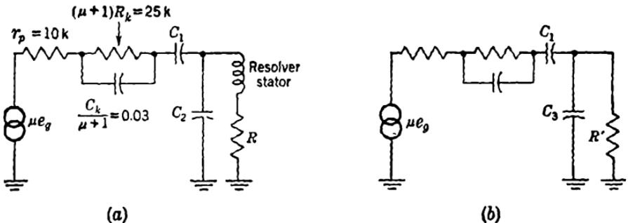
FIG. B-2.—Equivalent circuits of output stage.  $R'$  = apparent resistance of parallel-resonant circuit.  $C_3$  = excess of  $C_2$  over value required for resonant tuning. (a) Equivalent circuit of output stage; (b) simplified equivalent circuit if stator is tuned capacitatively.
