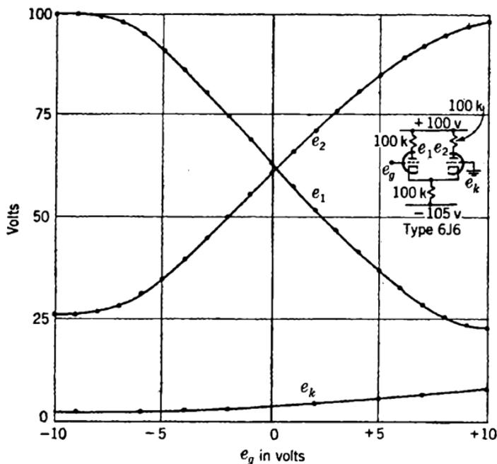
FIG. 11-29.—Example of differential amplifier and characteristic
