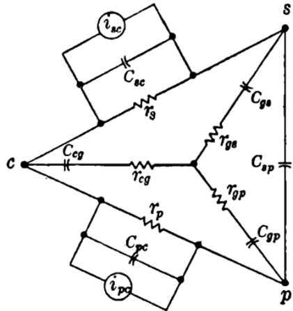
FIG. 12-14.—Representation of a pentode at moderately high frequencies.
