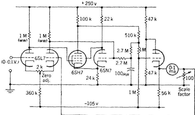
FIG. 11-63.—Voltmeter using high-gain amplifier.
