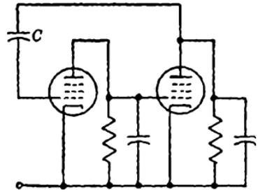
FIG. 2-15.—Negative-capacity circuit.
