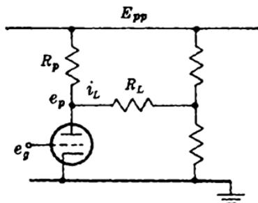
FIG. 11-32.—Plate as output terminal.
