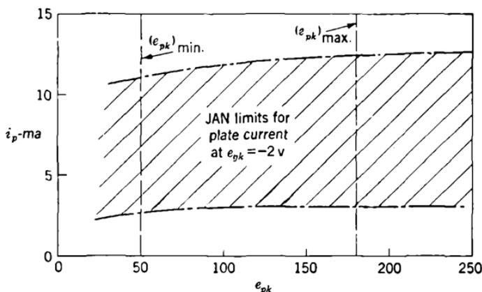
FIG. 9-16.—Type 6AK5 characteristic with tolerances.
