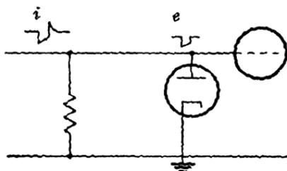
FIG. 3-14b.—Shunt diode.
