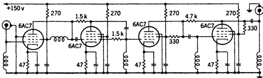
FIG. 6-18.—Flat quadruple feedback amplifier.
