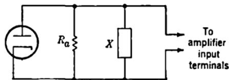
FIG. 14-4.—High-impedance diode noise generator.
