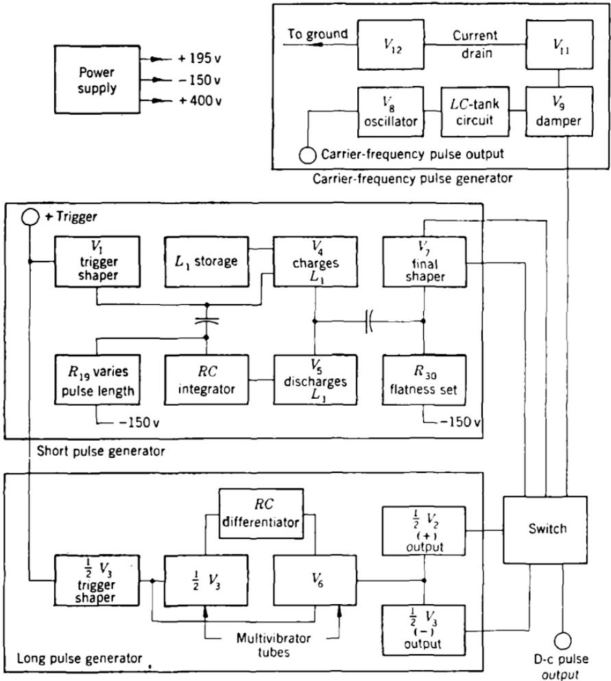
FIG. 8-4.—Block diagram of pulse generator.
