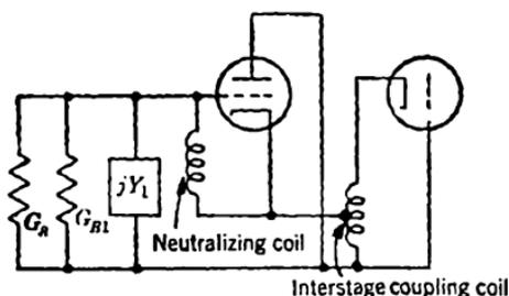
FIG. 13-17.—Grounded-plate-triode-grounded-grid-triode input configuration.
