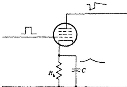
FIG. 3-3.—Cathode bypass circuit.
