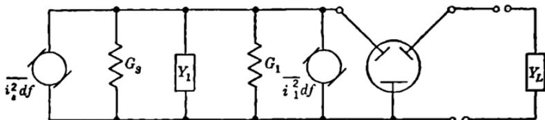
FIG. 13-2.—Equivalent circuit for input network.
