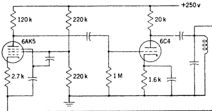
FIG. 9-20.—Driver circuit with tentative resistance values.
