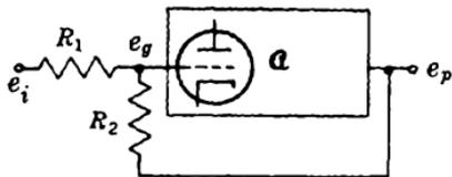
FIG. 11-51.—Direct feedback using resistance adding.
