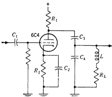
FIG. 9-13.—Output stage of driver.
