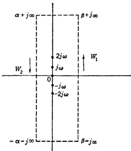
FIG. 1-21.—The  $\mathcal{S}$ -transform contour.
