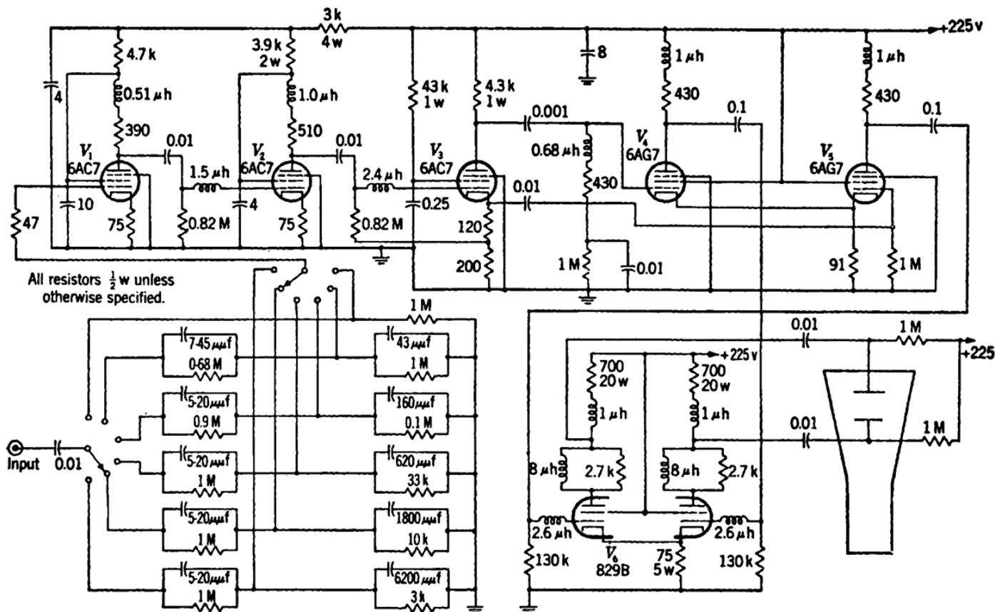
FIG. 2-38.—Pulse amplifier for deflection-modulated cathode-ray tube.
