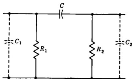
FIG. 3-24.—Coupling circuit including shunt capacity.
