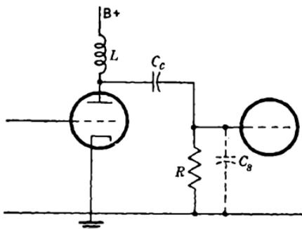
FIG. 3-10.—Choke-coupling circuit.
