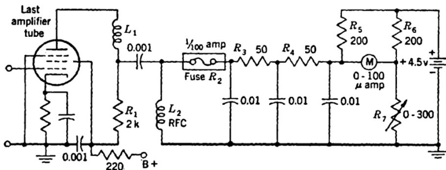
FIG. 14-16.—Unbalanced-bridge bolometer.
