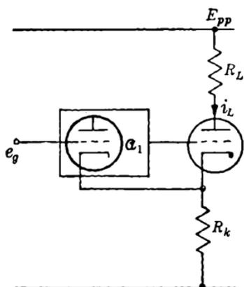
FIG. 11-54.—Cathode and screen feedback.
