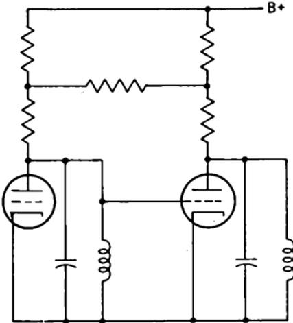
FIG. 6-15.—Feedback resistor tapped on load resistor.
