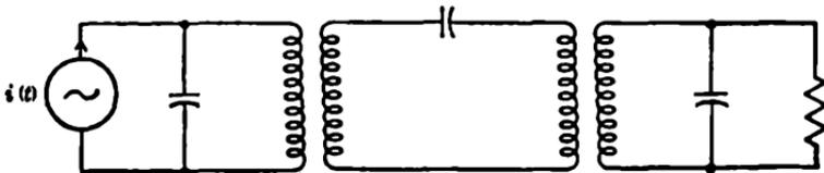
FIG. 1-6.—Network with three separable parts.
