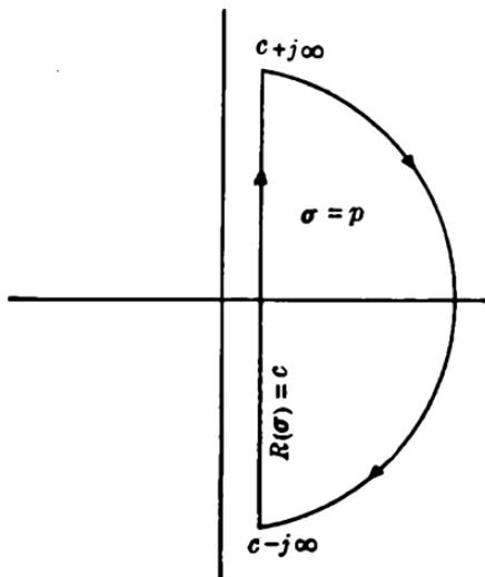
FIG. 1-15.—The infinite right-half circle.
