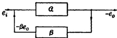
FIG. 10-4.—Block diagram of rudimentary feedback amplifier.
