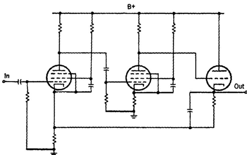
FIG. 2-22.—Simple illustration of over-all feedback.
