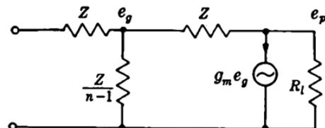
FIG. 2-30.—Nodal analysis of feedback-type mixer.
