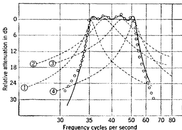
FIG. 10-16.--Pass band, four-section stagger-tuned filter. Calculated values, solid line; experimental values, dotted line. (a)  $f_1 = 40.6$  cps,  $Q_1 = 15$ ; (b)  $f_2 = 46.0$  cps,  $Q_2 = 6$ ; (c)  $f_3 = 54.9$  cps,  $Q_3 = 6$ ; (e)  $f_4 = 61.9$  cps,  $Q_4 = 15$ .
