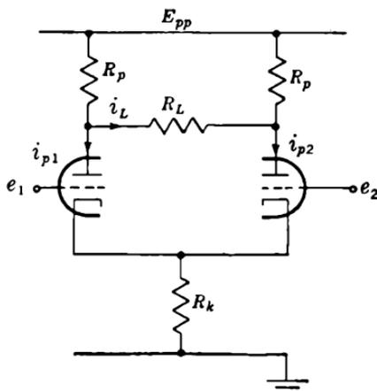
FIG. 11-36.—Differential amplifier with load.
