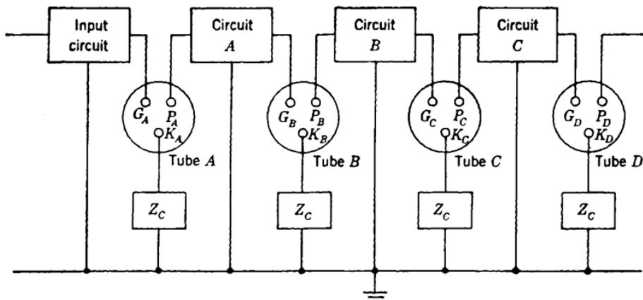
FIG. 8-13.—Tube and circuit line-up in an amplifier. The cathode-circuit impedance  $Z_c$  is a short circuit at the intermediate frequency and is equal to the bias resistance (50 to 200 ohms) at pulse and lower frequencies.
