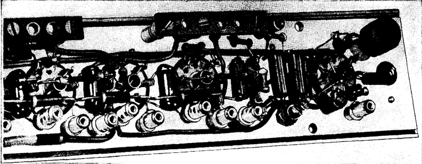
FIG. 6-20.—High-frequency inverse-feedback amplifier.
