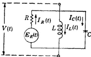
FIG. 12.3.—Thermal noise variables in  $RLC$  circuit.
