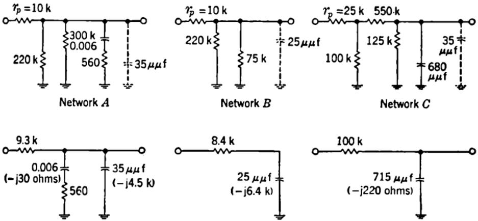
FIG. 9-38.—High-frequency stabilization networks with reactances at 1.0 Mc/sec.
