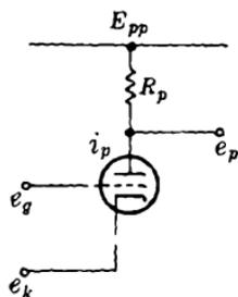
FIG. 11-24.—Triode with two input terminals.
