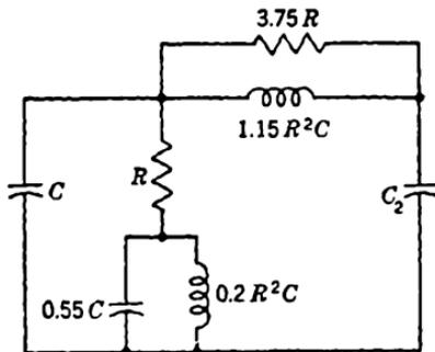
FIG. 2-8.—Four-terminal network designed for 1/1 capacity ratio.
