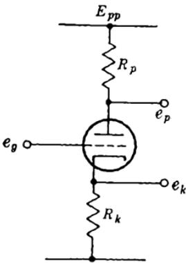
FIG. 11-12.—Triode with cathode and plate resistors.
