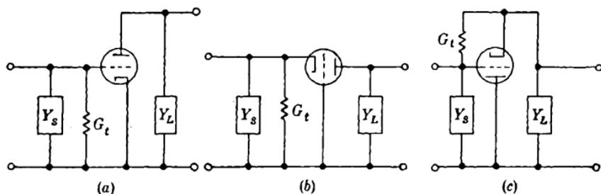
FIG. 13-5.—Alternative connections of first tube.
