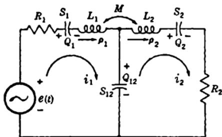
FIG. 1·7.—Two-mesh network.
