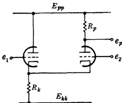
FIG. 11-25.—Cathode follower as an input means.
