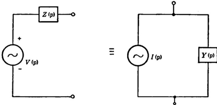
FIG. 1.1.—Voltage-current source equivalence.
