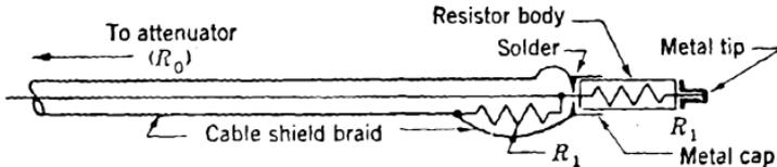
Fig. 8-11.—Dummy-crystal diagram showing approximate physical layout.
