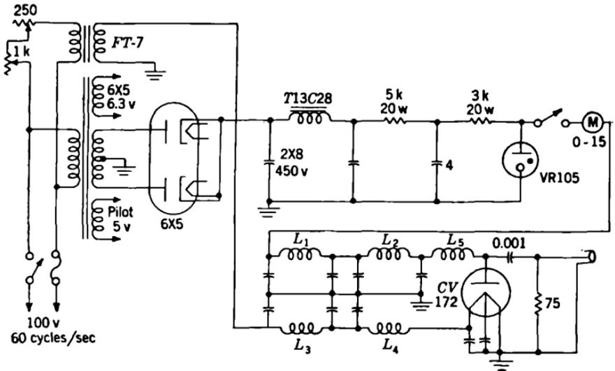
FIG. 14-9.—Circuit of noise generator.
