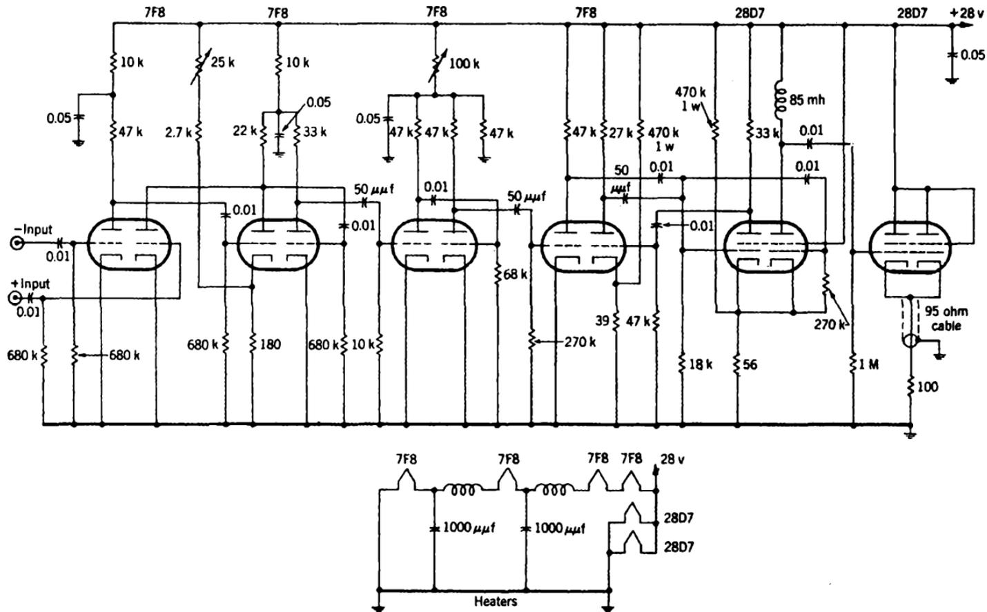
FIG. 3-44 —Circuit diagram of amplifier No. 4.
