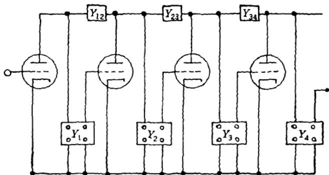
FIG. 6-3b.—Feedback chain using four-terminal shunt impedances.
