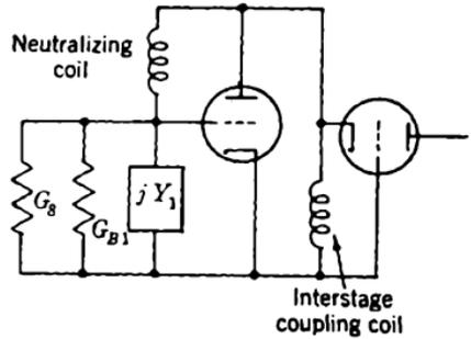
FIG. 13-12.—Grounded-cathode-triode-grounded-grid-triode input configuration.
