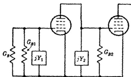
FIG. 13-9.—Grounded-cathode-pentode input circuit.
