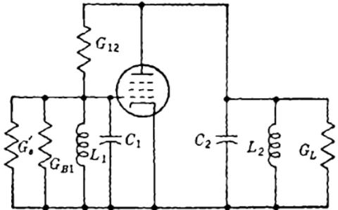
FIG. 13-20.—Pentode with plate-grid resistance feedback.
