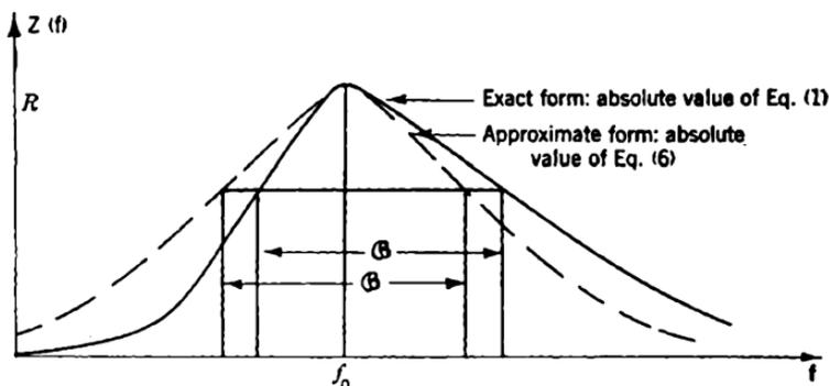
FIG. 4-3.—Resonance curve of single-tuned circuit.
