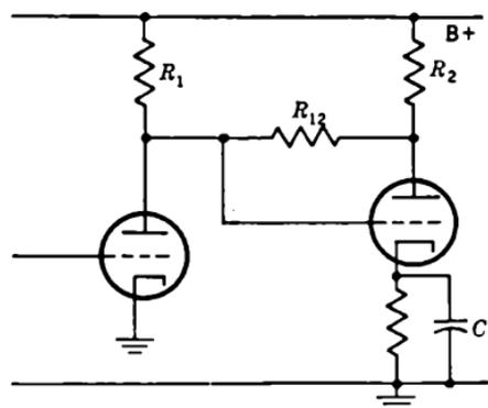
FIG. 3-22.—Direct-coupled inverse-feedback pair.
