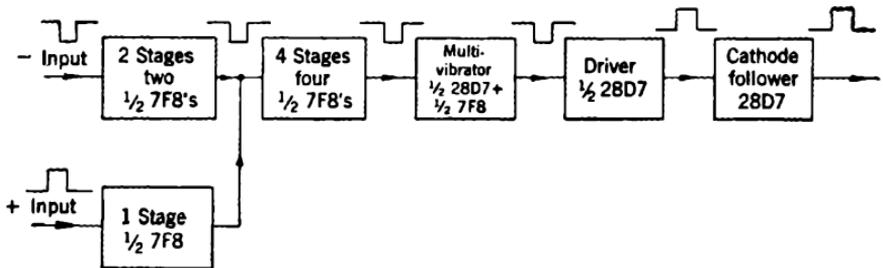
FIG. 3-43.—Block diagram of amplifier No. 4.
