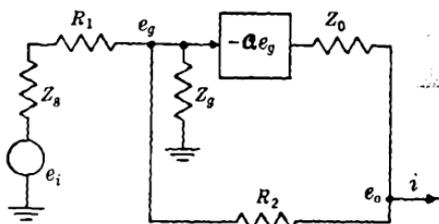
FIG. 9·2.—Schematic circuit for resistive-mixing feedback.
