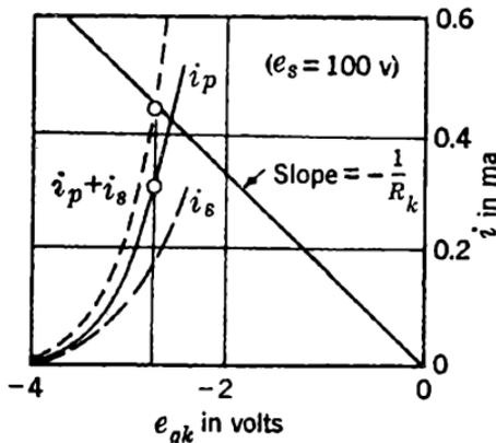
FIG. 11-74.—Determination of constant-current pentode current.
