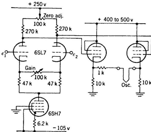
FIG. 11-64.—Two-stage oscillograph driver.
