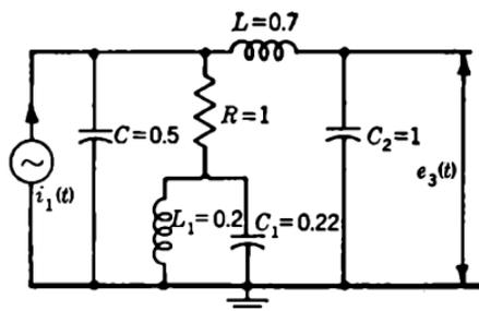
FIG. 1-26.—Four-terminal linear-phase coupling network.
