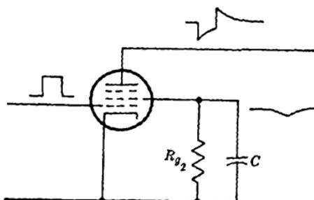
FIG. 3-4.—Screen bypass circuit.
