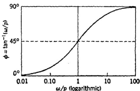
FIG. 9-5.—Inverse-tangent curve.
