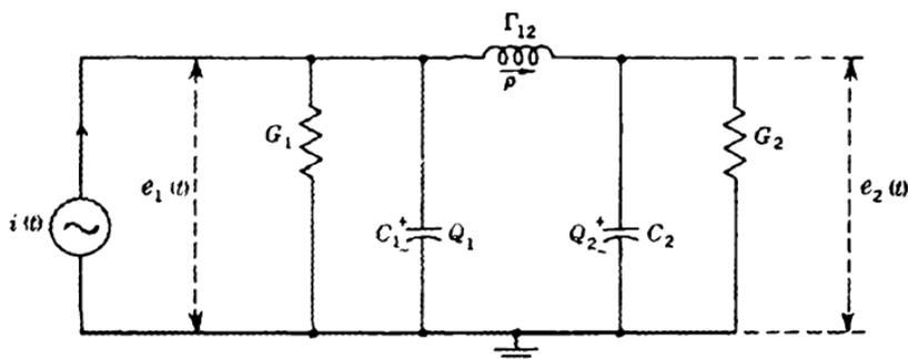
FIG. 1-16.—Two-node original network.
