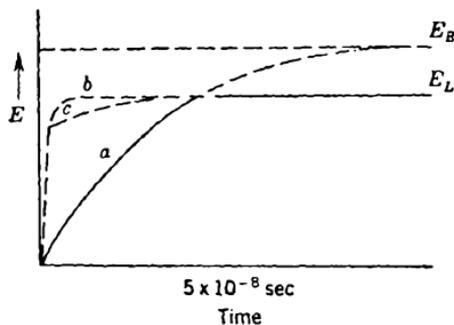
FIG. 8-7.—Shape of voltage rise at the  $V_4$ ,  $V_5$  junction. (a) Without compensating condensers  $C_{10}$  and  $C_{11}$ ; (b) compensating condensers set correctly; (c) compensating condensers too small.  $E_L$  is the voltage at which the grid of  $V_7$  starts to draw current.
