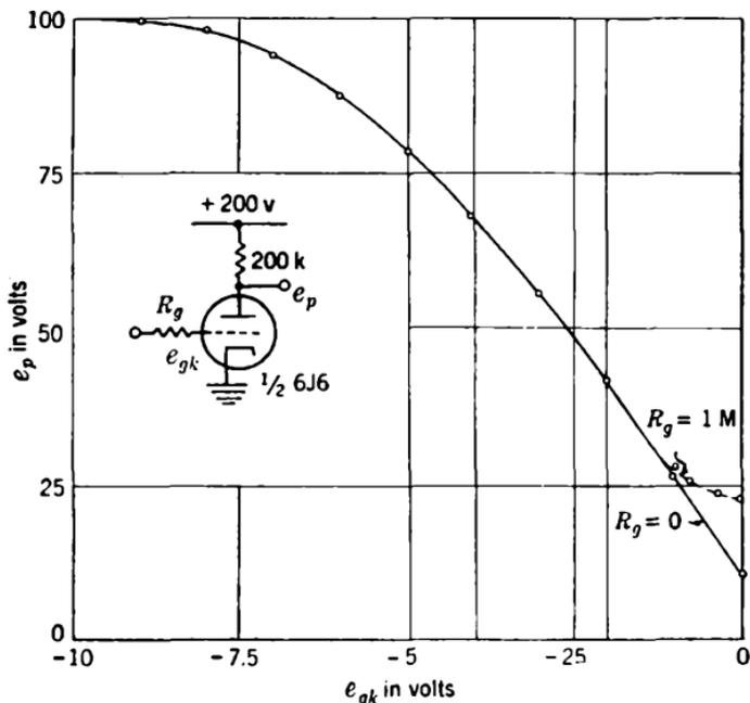
FIG. 11-11.—Typical triode amplifier characteristics.
