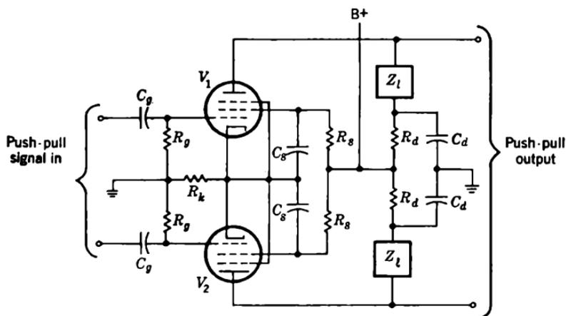
FIG. 2-34.—Typical push-pull pulse-amplifier stage.
