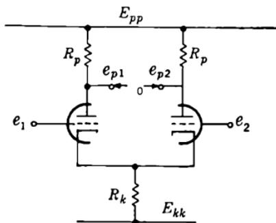
FIG. 11-28.—Symmetrical differential amplifier.
