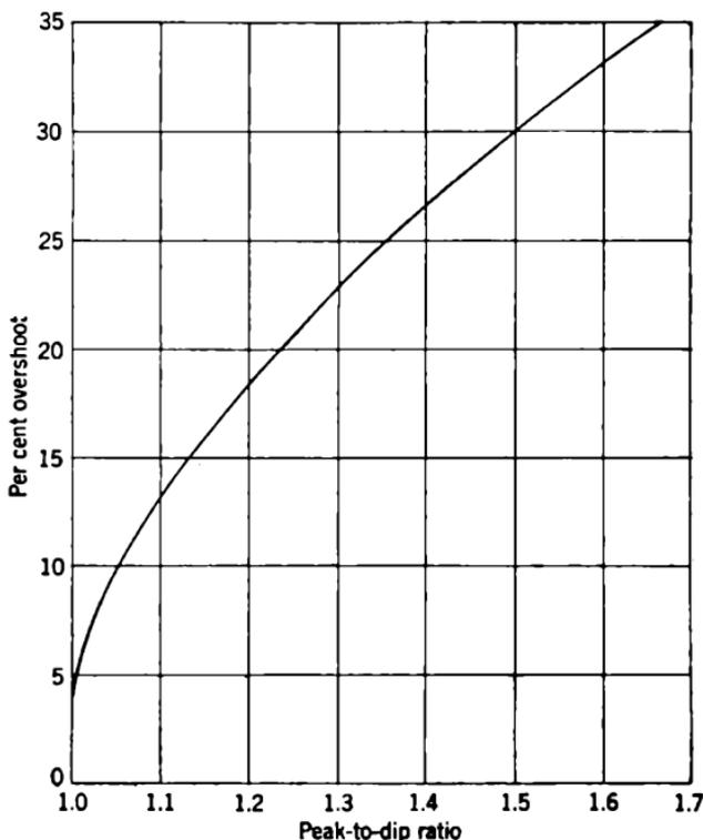
FIG. 7-4.—Overshoot of overstagged pair, as function of ratio of maximum response to response at midband. The curve also applies to double-tuned circuits of arbitrary  $Q$ -ratio, and inverse-feedback pairs.
