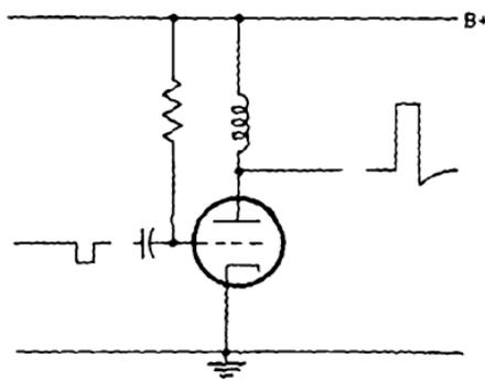
FIG. 3-29.—High-output voltage circuit.
