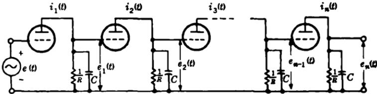
FIG. 1.23.—The  $n$ -stage RC-coupled pulse amplifier.
