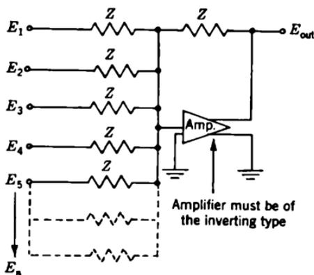
FIG. 2-29.—Feedback-amplifier mixer.
