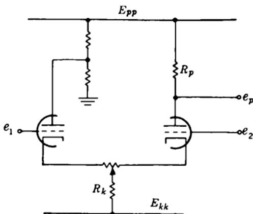
FIG. 11-27.—Method of zero adjustment.
