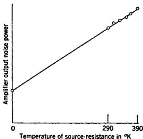
FIG. 14-17.—Radiometer determination of amplifier noise figure.
