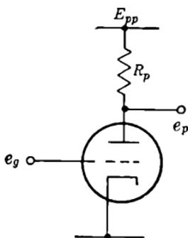
FIG. 11-9.—Simple triode amplifier.
