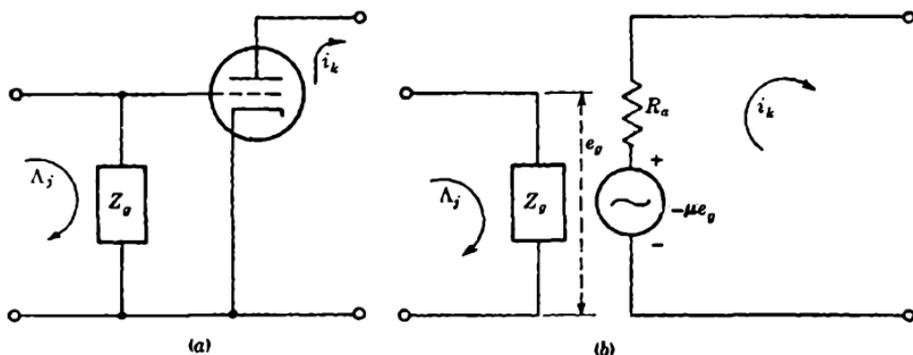
FIG. 1-9.—Equivalent circuit for a tube.
