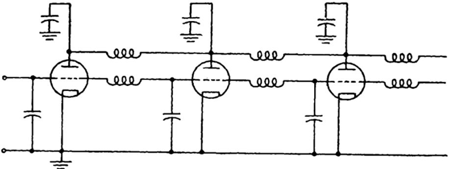
FIG. 2-16.—"Transmission-line" amplifier.
