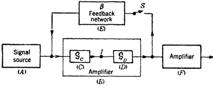
FIG. 13-18.—Block diagram of amplifier with feedback.
