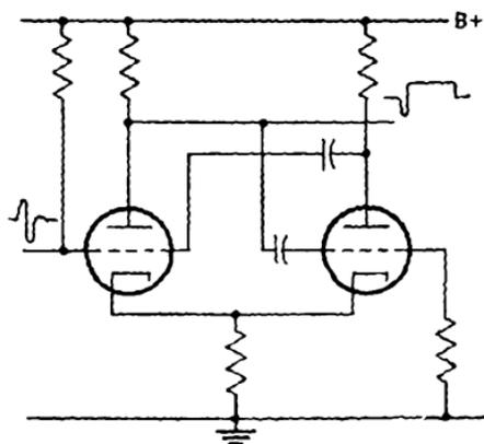
FIG. 3-28.—Multivibrator output circuit.
