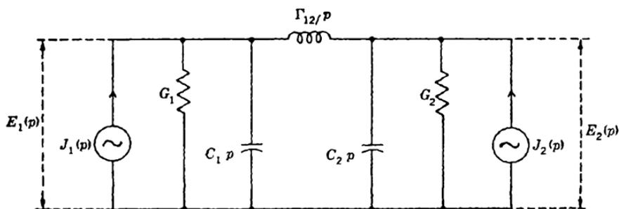
FIG. 1-17.—Two-node transform network.
