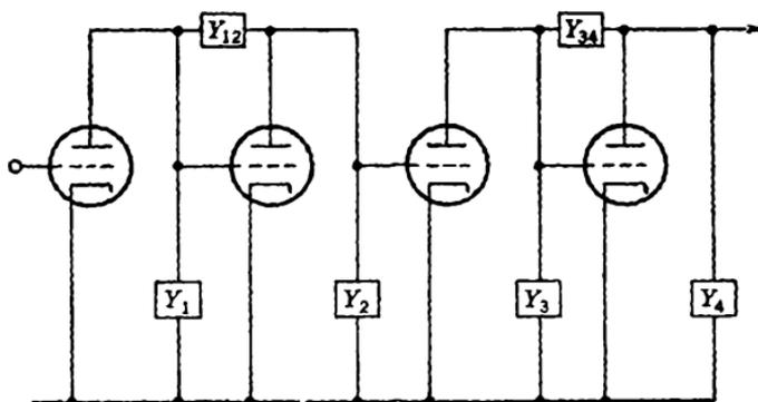
FIG. 6-4.—Feedback pairs.
