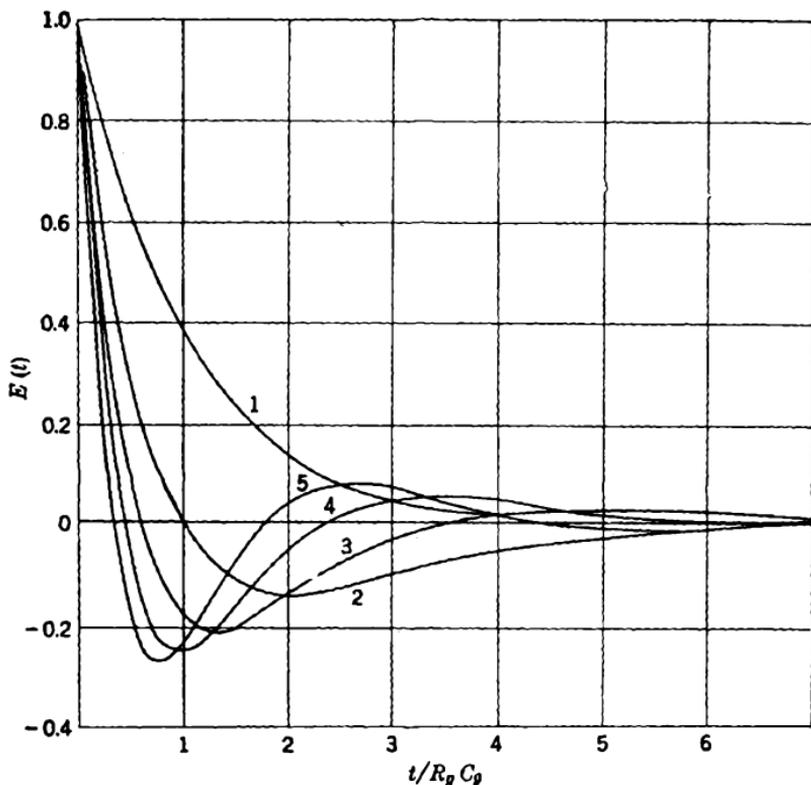
FIG. 2-17.—Step-function response of  $n$  capacitance-coupled stages each of time constant  $R_0C_0$ .
