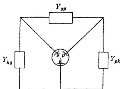
FIG. 13-6.—The general externally loaded three-node network.
