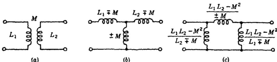
FIG. 1-11.—Transformer equivalent networks.
