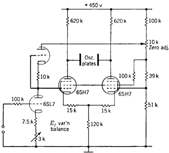
FIG. 11-67.—Two-stage voltage amplifier for oscilloscope deflection.
