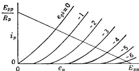
FIG. 11-10.—Plate characteristics with load line.
