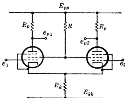
FIG. 11-31.—Pentode differential amplifier.
