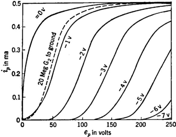
FIG. 11-49.—Plate characteristics of a 6V6 triode.
