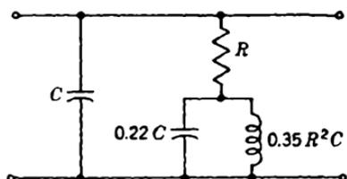
FIG. 2-6.—Two-terminal linear-phase network.
