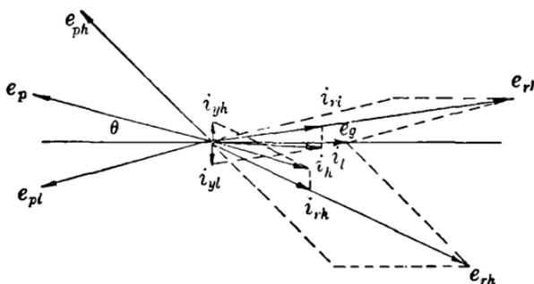
FIG. 6-12.—Vector diagram off resonance showing transit-time effect.
