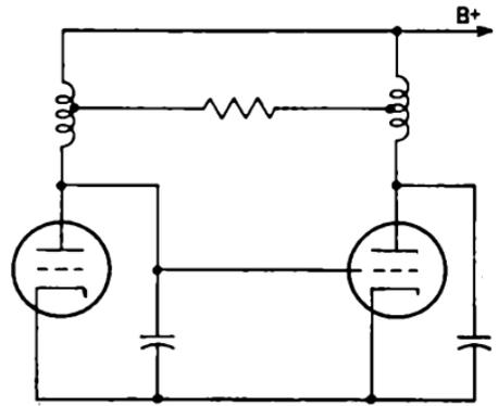
FIG. 6-17.—Feedback resistor tapped on coil.
