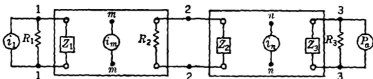
FIG. 12-16.—Two component networks in cascade.
