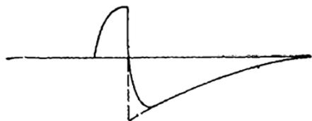
FIG. 3-11.—Overshoot produced by choke-coupling circuit.
