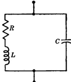
FIG. 2-4.—Shunt-peaked circuit.
