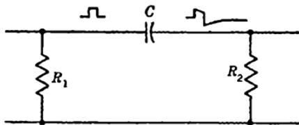
FIG. 3-1.—Coupling circuit.
