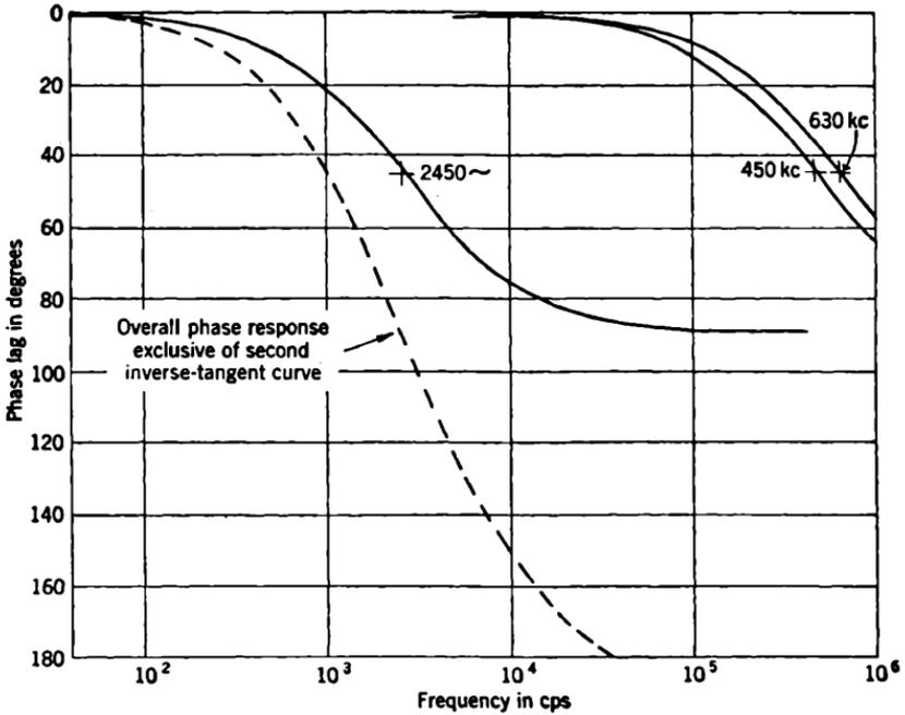
FIG. 9-35.—Calculated phase characteristics of high-frequency network.
