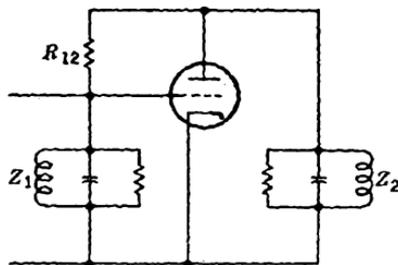
FIG. 6-2.—Simple feedback stage.
