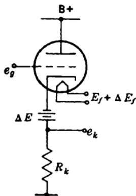
FIG. 11-40.—Heater-voltage variation effect on a cathode follower.
