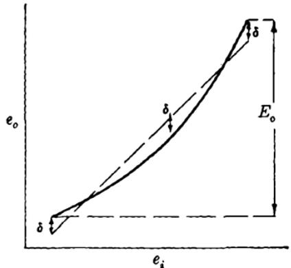
FIG. 11-52.—Relation of nonlinearity to change of gain.
