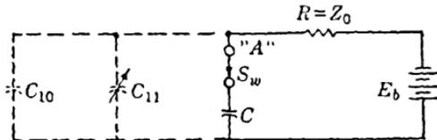
FIG. 8-6.—Equivalent circuit of delay line after firing of  $V_4$ . Before the firing of  $V_4$ , represented by the switch  $S_w$ , the voltage across  $C$  is zero and the voltage across  $C_{10}$  and  $C_{11}$  is the supply voltage  $E_b$ . When  $S_w$  is closed, the charge on  $C_{10}$  and  $C_{11}$  is rapidly redistributed and shared by  $C$ .
