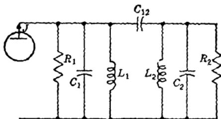
FIG. 5-1b.—Capacity-coupled double-tuned circuit.
