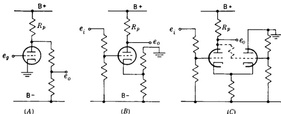
FIG. 11-33.—Voltage output embracing ground potential.
