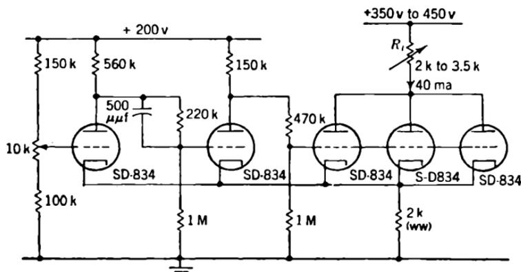
FIG. 11-66.—Current-regulating d-c amplifier.
