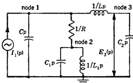
FIG. 1-27.—Transform of the network of Fig. 1-26.
