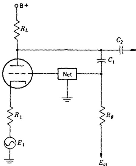
Fig. 10-8.—Single-stage frequency-selective amplifier.
