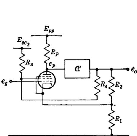
FIG. 11-55.—Example of current feedback.
