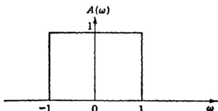
FIG. A-3.—Idealized low-pass filter  $A(\omega) = 1$  for  $-1 < \omega < 1$ ,  $= 0$  otherwise.
