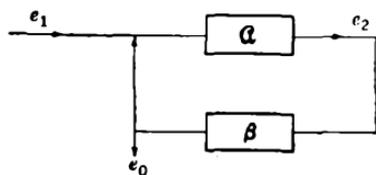
FIG. 10-7.—Block diagram of rejection amplifier.
