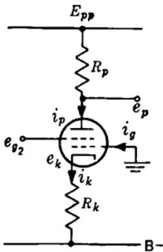
FIG. 11-48.—First grid as diode plate.
