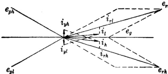
FIG. 6-10.—Vector diagram off resonance.
