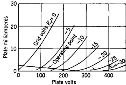
FIG. 9-28.—D-c operation of third amplifier stage.
