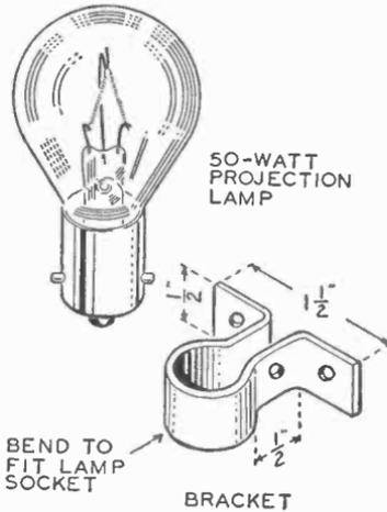
PROJECTION LAMP. SOCKET, RESISTOR AND HOMEMADE BRACKET FOR LIGHT SOURCE
