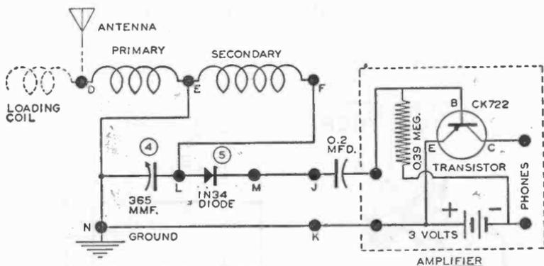
**SCHEMATIC CIRCUIT DIAGRAM SHOWING HOW TO CONNECT THE AMPLIFIER TO THE "MORE SELECTIVE" CRYSTAL RECEIVER DESCRIBED IN CHAPTER III**
