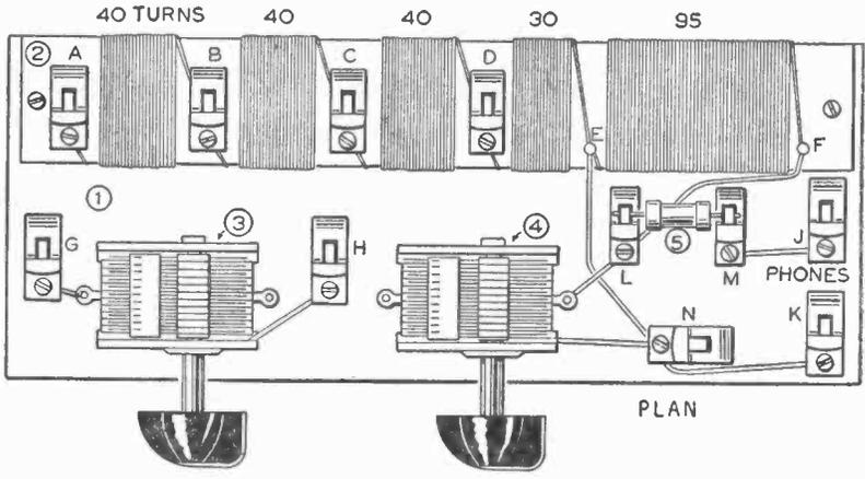
**PLAN OF THE CRYSTAL RECEIVER AND DETAILS OF THE TUNING INDUCTANCE**
