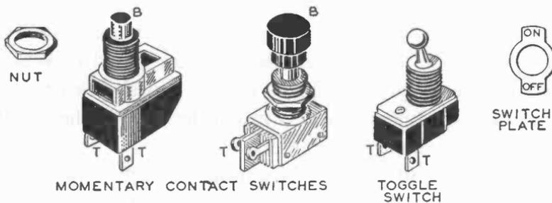
**SWITCHES OF THE TYPES USED IN BUILDING THE SNIFFER**
