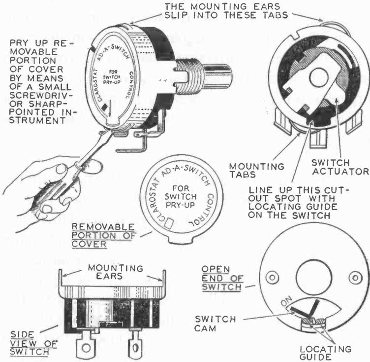
**HOW TO ATTACH AN "ON-OFF" SWITCH TO A CONTROL**
