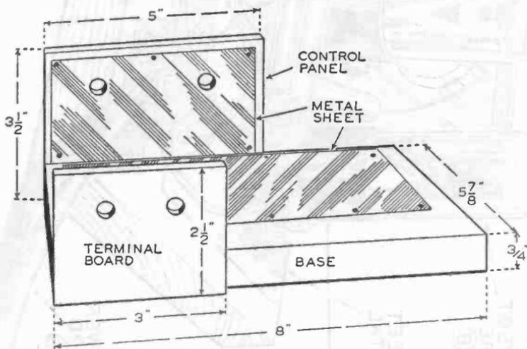
THE CHASSIS UPON WHICH THE COMPONENTS OF THE AMPLIFIER ARE MOUNTED
