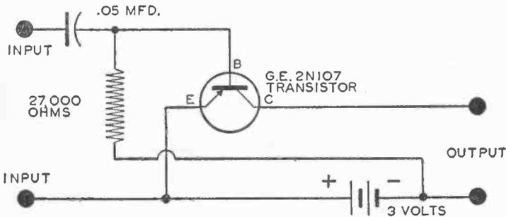
**SCHEMATIC CIRCUIT DIAGRAM OF
