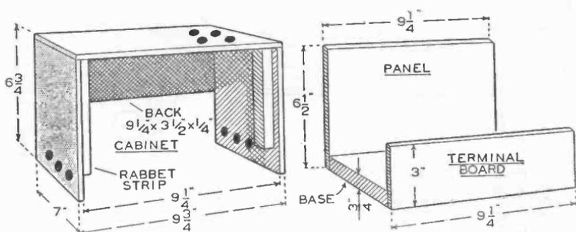
**CABINET AND CHASSIS FOR AN ENCLOSED MODEL OF THE AMPLIFIER**
