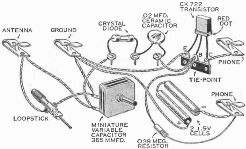
**HOW TO BUILD A TRANSISTOR
