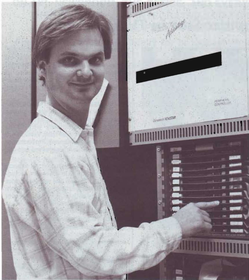
CFPL-TV's Brian Fox points to Newstar system co-processor cards, each of which handles two Zentec terminals. — Photo by Keith Risler
