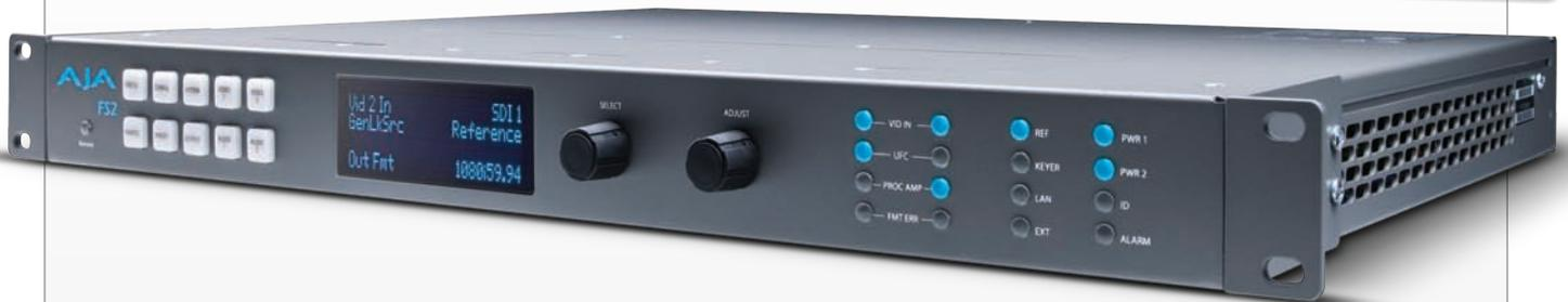
FS2 delivers dual-channel conversion and frame synchronizing power and flexibility in a slim 1RU space. With two independent video and audio processors, FS2 can do the work of two separate devices or combine both processors together for maximum flexibility.
