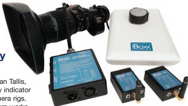
The new Boxx tally system works with any broadcast camera that uses a standard 12 pin Hirose lens cable.
