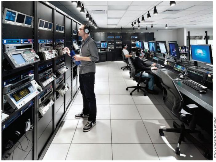
The Ingest Room at Corus Quay handles as many as 70 signals all told, with intake and delivery of several individual linear individual channels and multiple digital media formats. Photo credit: Richard Johnson
