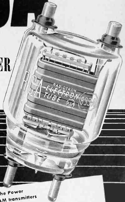
The RCA 833-A, the Power Triode for 1 Kw AM transmitters
