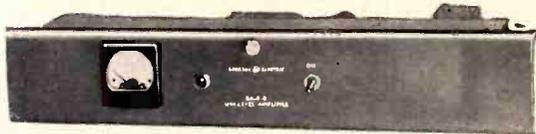
For Audio Gain Control Uni-Level Amplifier BAC-9-B
