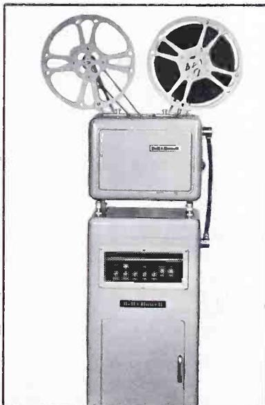
16mm TV Jan film chain projector Model 614EVMS combining excellent picture and sound quality with long life design—features optical and magnetic playback, choice of lenses, air cooled aperture, lower loop restorer, separate drive motors and local or remote control.
