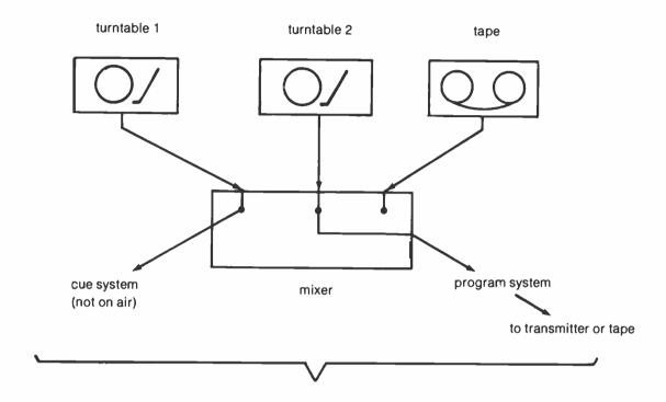
Turntable 2 is playing record which is on-air. Operator can set up record on turntable 1 by listening to it on "cue" system.
