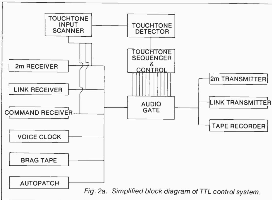
Fig. 2a. Simplified block diagram of TTL control system.
