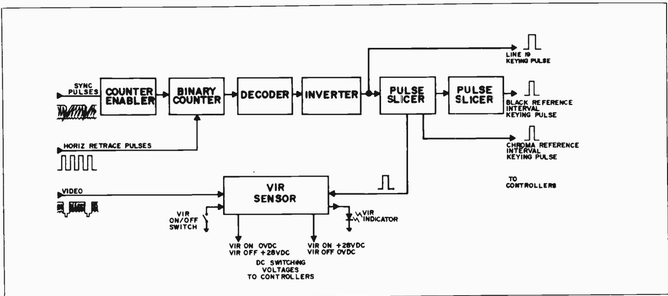
Fig. 3. Block diagram of the line recognizer circuitry
