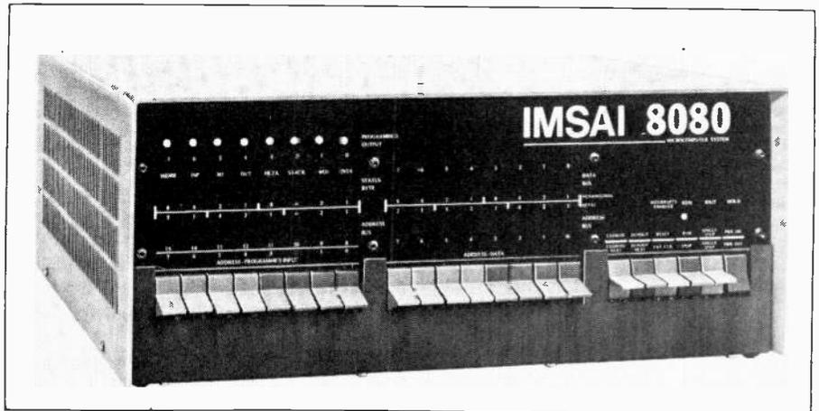
Fig. 2. The control panel on this IMSAI 8080 has LEDs to display the address bus, the data bus, and a programmed output, and switches to input addresses and data. There are also switches and LEDs to control and display the status of the processor.
