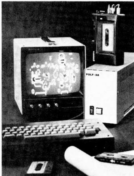
Fig. 3. The Poly-88 is a 'front-panel-less' computer and uses a built-in VDU to control its operation.
