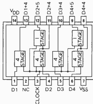
**CD4009A, 4049A HEX BUFFER CONVERTER — INVERTING**
