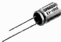
pling, decoupling, bypass, filtering. Excellent capacitance stability. Low leakage current, low ESR. Metal-encased, with plastic insulating sleeve. Capacitance values from .47 to 3300  $\mu$ F. Voltage ratings from 6.3 to 63 WVDC.
