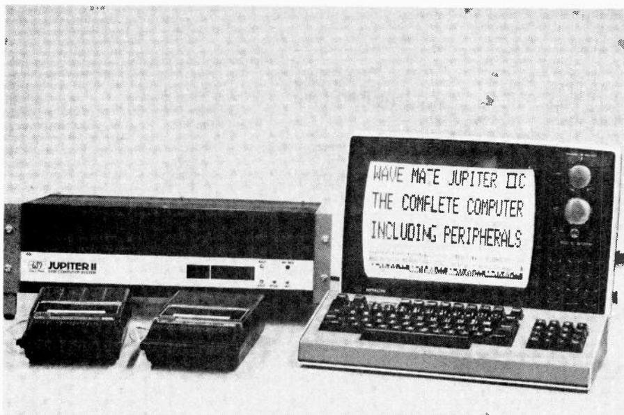
Fig. 5. The Jupiter II is a 6800-based computer built using wire-wrap cards. Again, a VDU is the prime method of communication with the computer.
