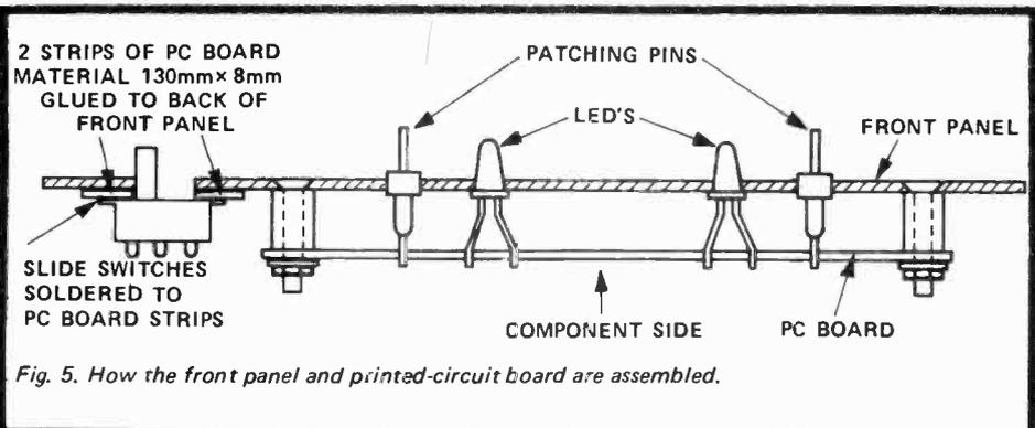
Fig. 5. How the front panel and printed-circuit board are assembled.
