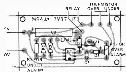
Component Overlay — Alarm with Relay
