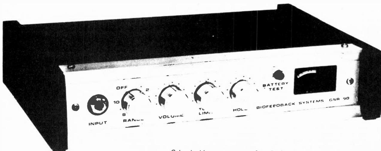
Galvanic skin response meter from Biofeedback Systems. A large external meter may be added to this unit.
