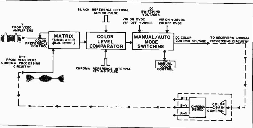
Fig. 6. The colour control circuitry is similar to the tint controller
