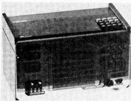
Fig. 6. The keyboard-and-display approach is illustrated by this EPA Micro-68 (shown here in its expanded form).
