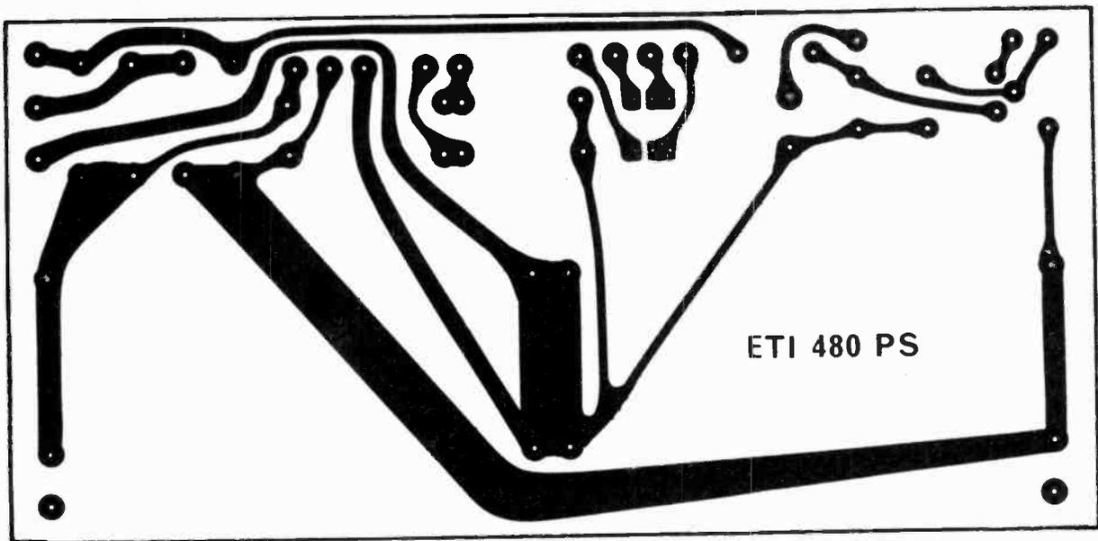
Printed circuit layout of the power supply. Full size 160mm x 76mm.
