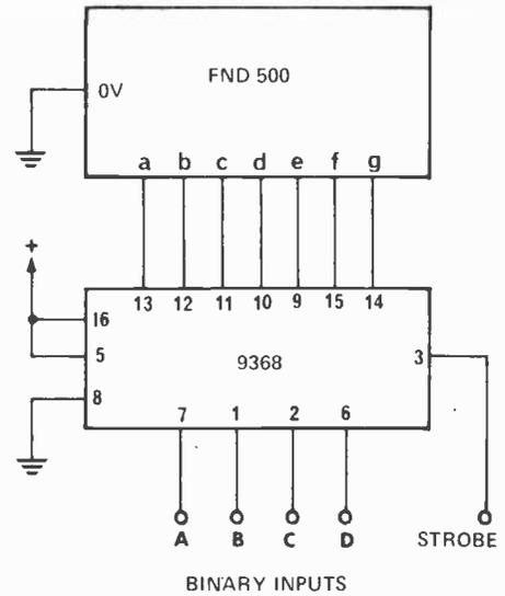
The circuit diagram of one half of the display.
