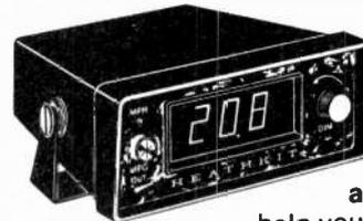
The **NEW CI-1078 digital electronic Miles-per-Gallon Monitor/Speedometer** reads 0.99 mpg, 0-99.9 mph in an orange-amber digital readout. It will help you drive more efficiently, save gas and money too!
