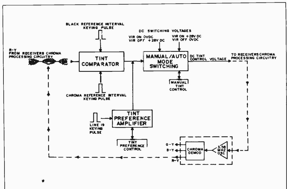
Fig. 4. The VIR tint controller stages from a closed loop feedback system
