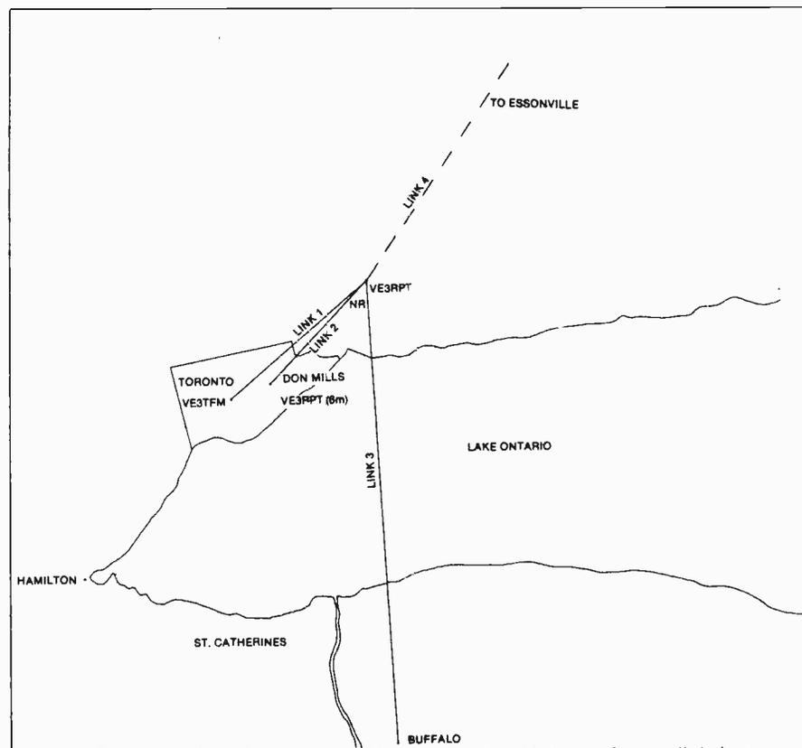
*Fig. 3 Southern Ontario repeater sites and links. Link 1 - 2 way link between VE3RPT & VE3TFM, used for Autopatch only. Future use includes inter-repeater signalling. Link 2 - One-way link from VE3TOR TO VE3RPT. Feeds signals received on 52.76 MHz up to main Tx on 52.525 MHz. Link 3 - 2 way link to the Buffalo repeaters. Link 4 - Proposed link will give Toronto users access to VE3TBF, Essonville and one repeater in Ottawa.*
