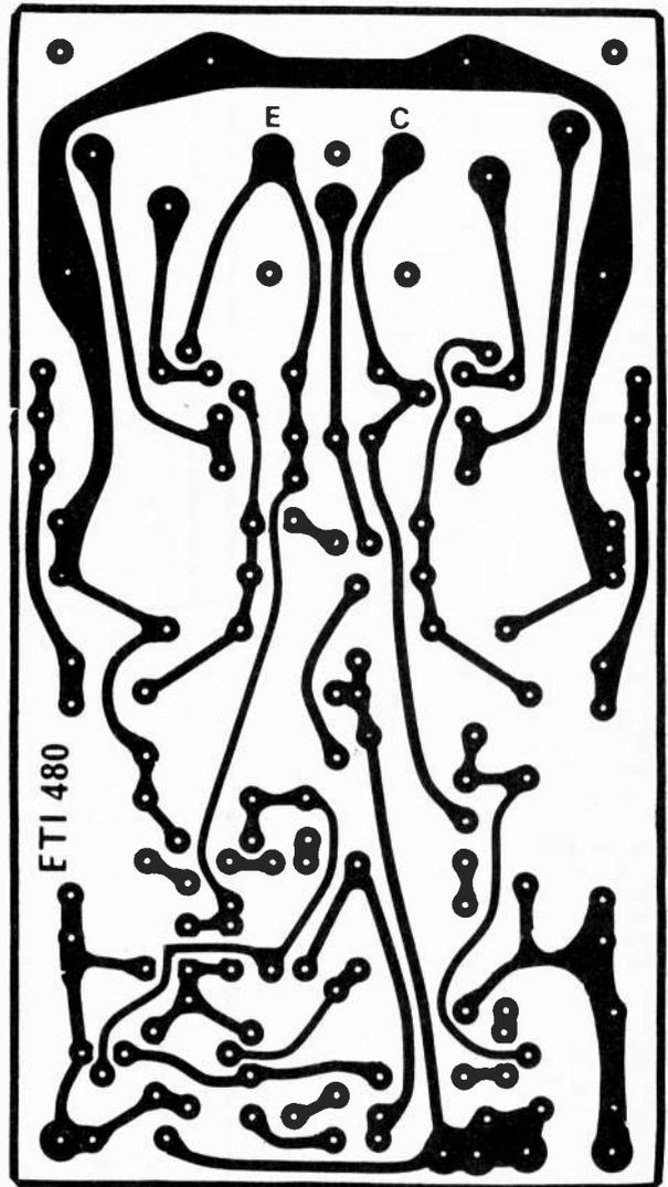
Printed circuit layout of the amplifier. Full size 140mm x 76mm.
