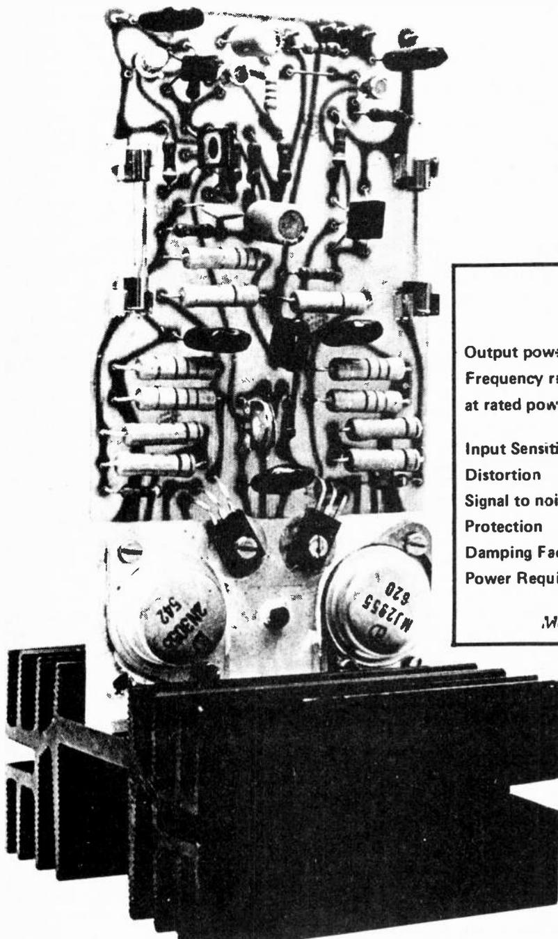
The screws holding the 2N3055/MJ 2955 should also be insulated where they pass through the heatsink bracket. The BD 139 and BD 140 do not need any insulation other than the mica, provided 3mm screws are used. In the 100W version the additional transistors are mounted on the heat-sink bracket outside the PC board area.
