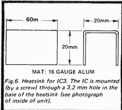
Fig. 6. Heatsink for IC3. The IC is mounted (by a screw) through a 3.2 mm hole in the base of the heatsink (see photograph of inside of unit).
