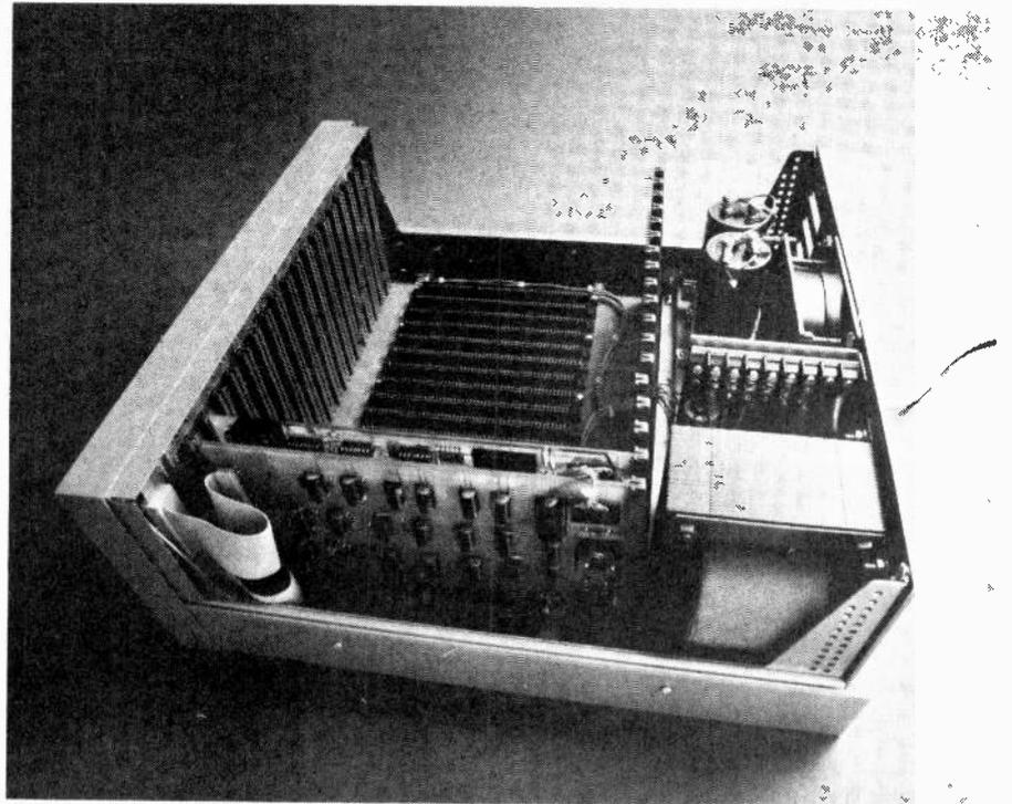
Fig. 1. This Altair 8800b shows the internal construction of a microcomputer. Note the heavy duty supply and the card slots, both designed for easy expansion.
