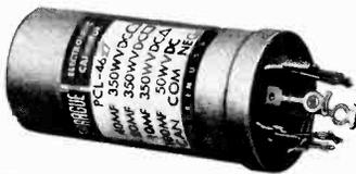
surge voltages, high ripple currents, high temperatures. Etched cathode construction. Ideal for selenium rectifier circuits. Single, dual, triple, and quadruple section units. Capacitance values from 2 to 3000  $\mu$ F. Voltage ratings from 3 to 500 WVDC.
