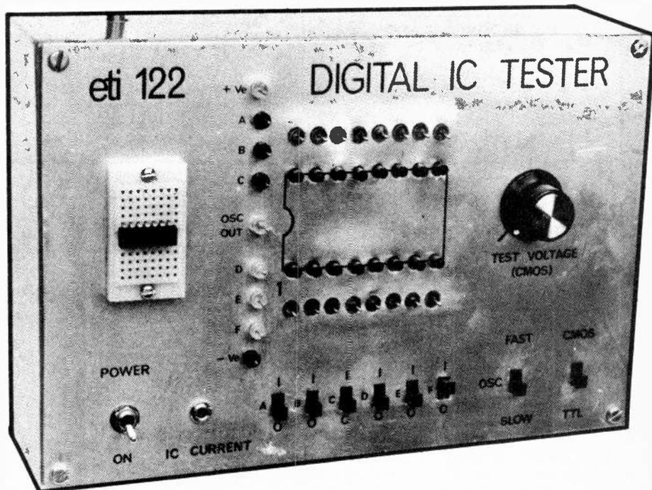
EXPERIMENTERS often damage ICs in the process of developing a new circuit and often try a new IC in a circuit that is not working to eliminate that as a possible cause. The result of this is that one usually finishes up with a box full of ICs which are of dubious value. To sort out these ICs one must use a tester that is capable of testing the wide range of differing ICs that are available in the most commonly used families.
