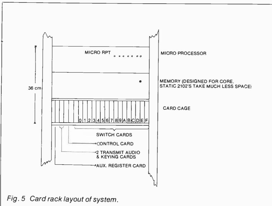
Fig. 5 Card rack layout of system.
