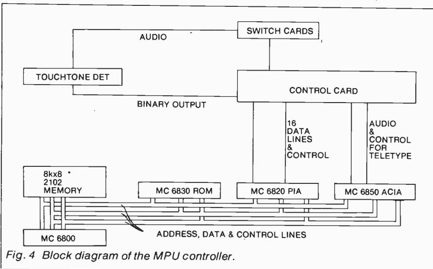
Fig. 4 Block diagram of the MPU controller.
