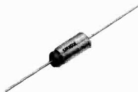
circuitry, especially where high volumetric efficiency, low cost, and dependable performance are important considerations. Metal-encased, with plastic insulating sleeve. Capacitance values from 1.5 to 3300  $\mu$ F. Voltage ratings from 3 to 100 WVDC.
