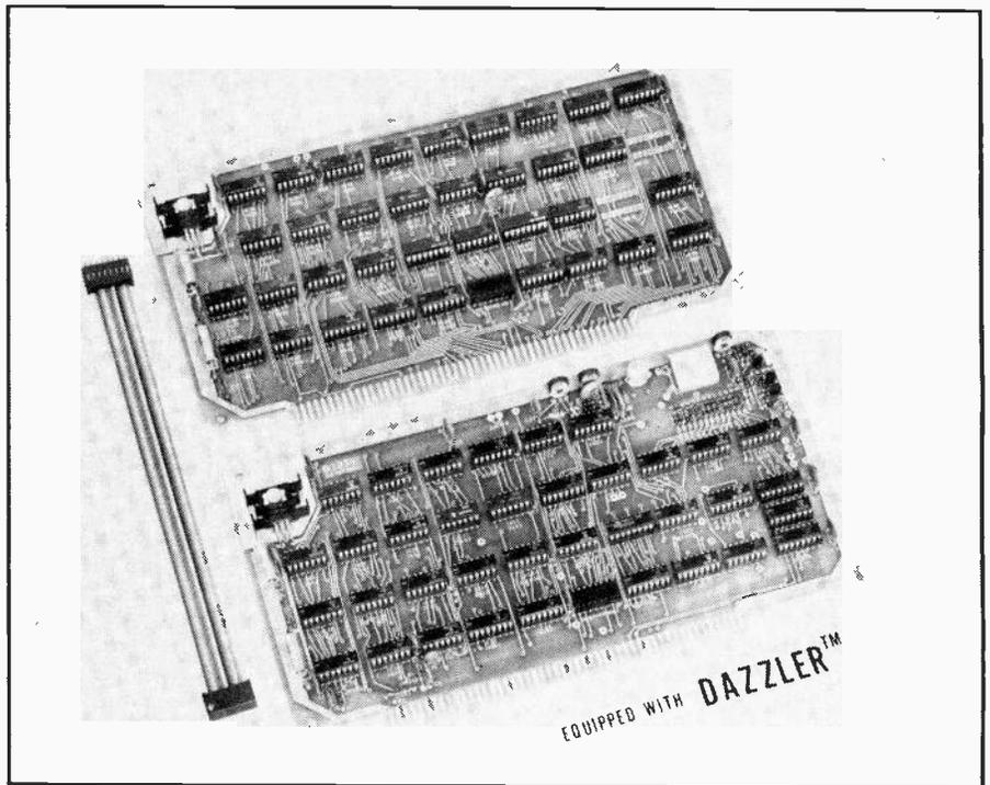
Fig. 4. Cromemco's Dazzler is a colour VDU for graphic computer games, like the smaller TV games chips but many times more versatile. It is built on two S-100 bus compatible cards and so fits several computers.
