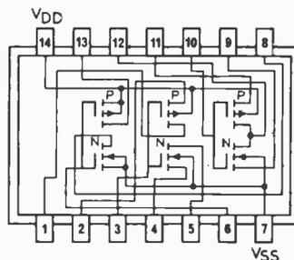
**CD4010A, 4050A HEX BUFFER CONVERTER — NON-INVERTING**
