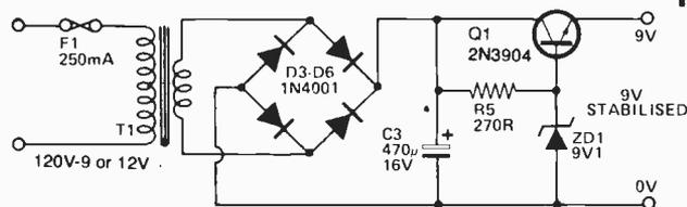
Temp Alarm Power Supply Circuit
