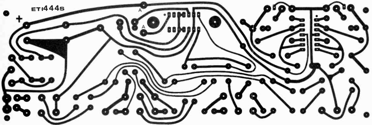
As we mentioned last month, National Semiconductor have changed the package of the LM379. Here is the revised PCB layout which fits the LM379S, which most readers will find easier to obtain. Our thanks go to Canmos Electronics for their assistance with this.
