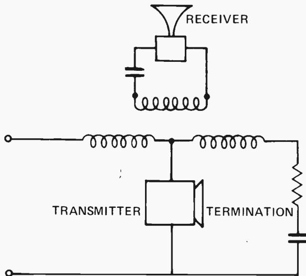
Fig. 1. How a Hybrid coil stops you from talking to yourself.
