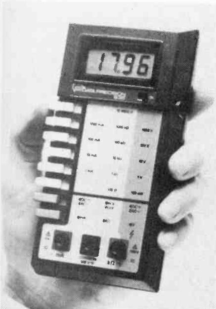
The meter offers 20 ranges of DC or AC voltage and current and resistance measurements, including both high and low resistance excitation capability. Ranges, functions, and excitation level are selected using pushbutton switches, allowing one-handed operation. Measurements including appropriate polarity sign and decimal points and a warning indicator for low battery voltage are displayed on a 3½ digit, 0.5" high, liquid crystal display.
