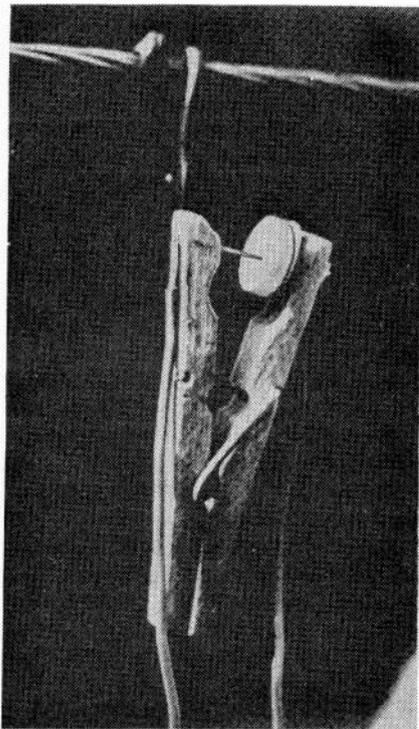
Vertically suspended hygroscopic transducer features disposable actuating element.
