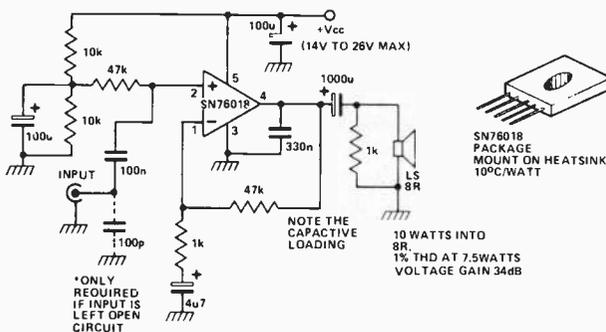
This is a very simple and inexpensive monolithic power amplifier made by Texas Instruments. It comes in a package that looks like a plastic power transistor with five legs.
