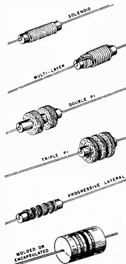
Fig. 1. General range of constructor styles of RF chokes. The particular style employed depends on the required or allowable component. Size, the inductance, the application and the required characteristics.
