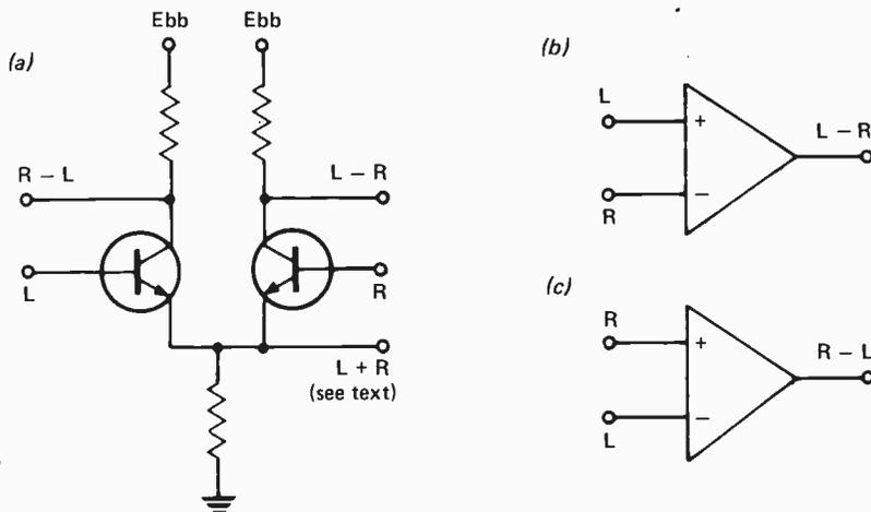
Fig. 4. Extracting Difference Signal. (a) Differential Amp. (b) and (c) Block diagram of differential amps.
