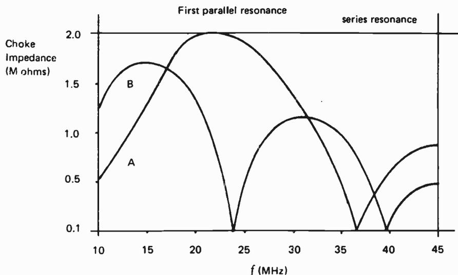
Fig. 4. Typical behavior of two RF chokes (A = around  $10 \mu\text{H}$ , B = around  $40 \mu\text{H}$ ) over a range of frequencies.
