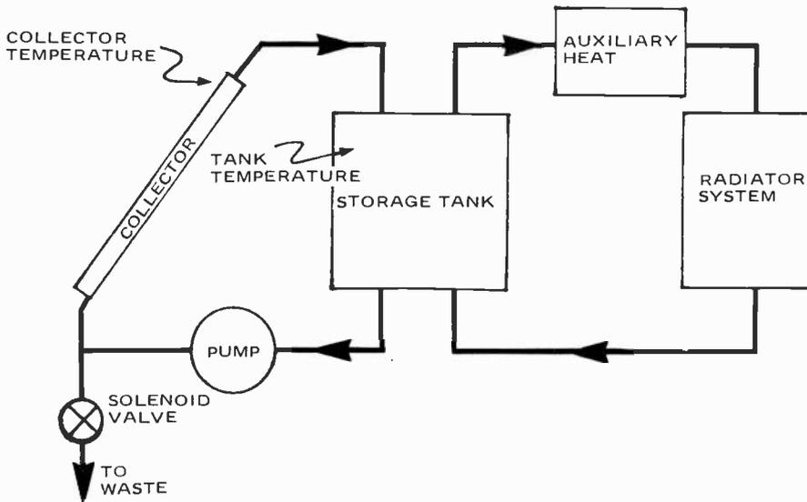
Fig. 2. Space Heating. A radiator system is shown here. This is essentially similar to the water heating system shown in Fig. 1.. However, it is not necessary to keep the two liquids apart. Thus, as long as your collector liquid is compatible with your rads, the tank can simply be a common storage tank for both circuits. The control system is similar to that of Fig. 1. as are the commonly used turn-on and turn-off differential figures.
