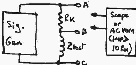
Set the signal generator to some frequency, keep trying new values of  $R_k$  until voltage between B and C equals voltage between A and B. If  $R$  has to be very large, then reduce frequency, if it has to be very small then increase frequency.
