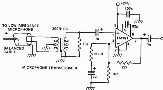
Professional audio equipment generally uses balanced inputs and outputs. This means that the inputs and outputs are differential, which is usually obtained by having balancing input and output transformers.
