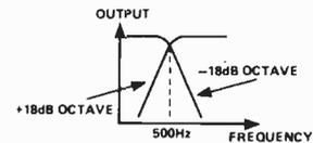
The circuit shown is for a two speaker system having a crossover frequency of 500 Hz. The filter structures are third order Butterworth multiple feedback, low pass and high pass. (Third order implies that roll off slopes of  $\pm 18$  dB/octave are obtained.)
