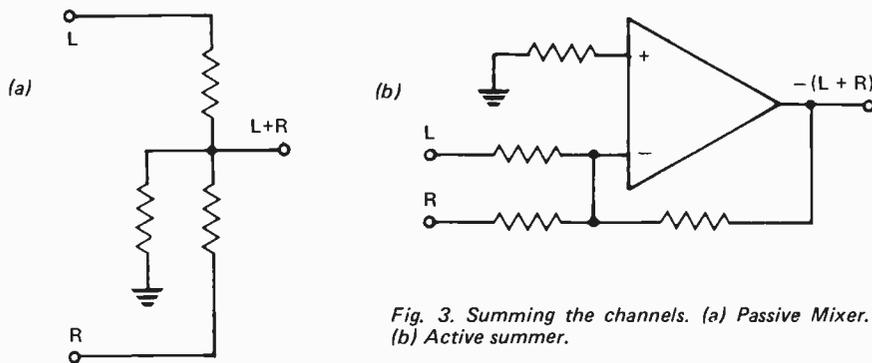
Fig. 3. Summing the channels. (a) Passive Mixer. (b) Active summer.
