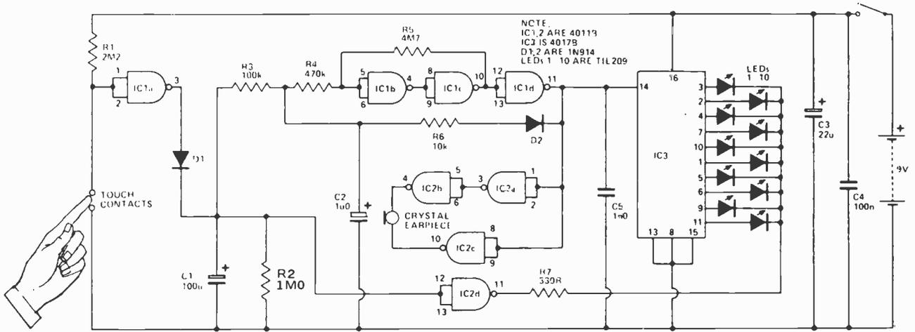
Fig. 1. Circuit diagram of the Wheel of Fortune.
