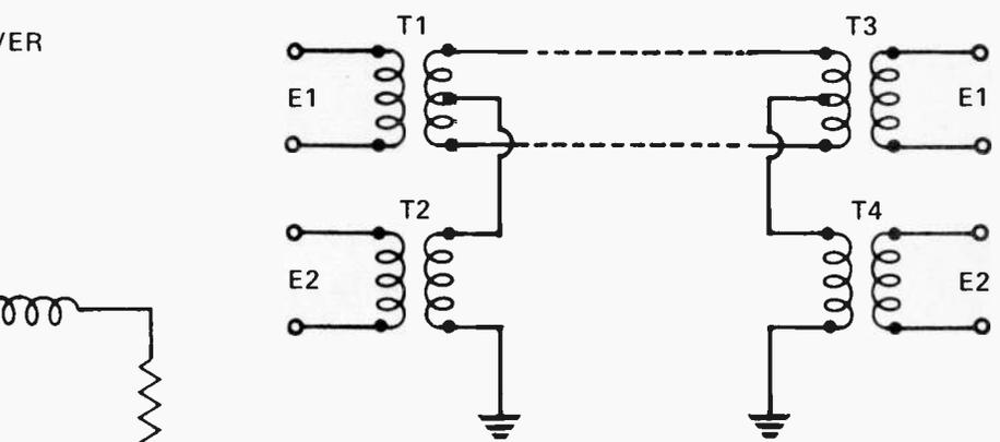
Fig. 2. Basic Simplex circuit, sometimes called "Phantom". Originally used in opera broadcasts.
