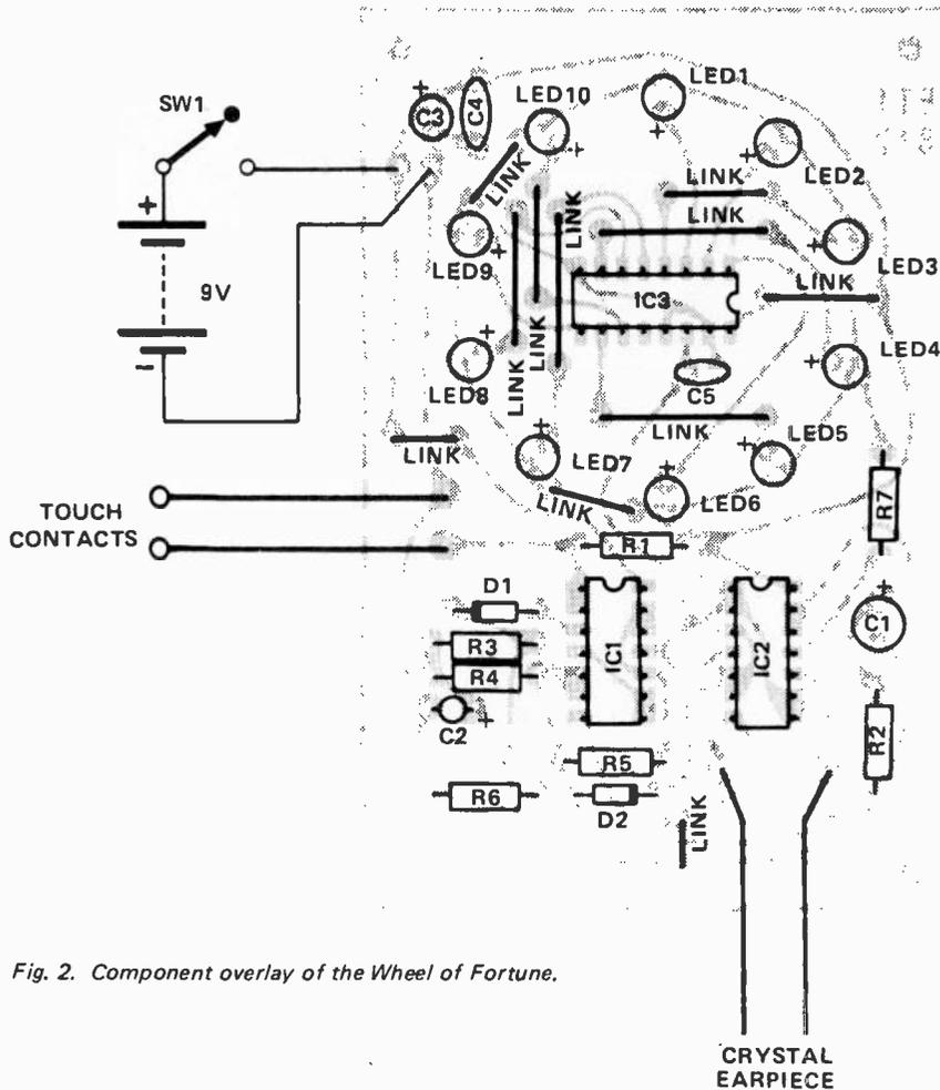
Fig. 2. Component overlay of the Wheel of Fortune.
