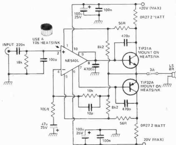
An audio power amplifier can be constructed from a power driver op amp plus a pair of transistors. The power driver is a NE540 made by Signetics. It generates quite a bit of internal heat and so a T05 heat sink is required. Note that this design uses five stabilizing capacitors.
