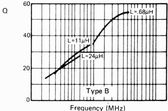
Fig. 7. Typical Q values versus frequency for several values of two different sizes of moulded RF chokes (From IRH). A = 6.4 mm dia. x 78 mm long. B = 6.4 mm dia. x 27 mm long.
