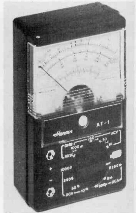
The Hansen AT-1 is a mini-sized multi-meter 'designed as the subsidiary instrument' for engineers and technicians. It features protection against magnetic interference, 90 degree mirrored scale, and ABS case. GE diodes give a good frequency response on AC volts ranges.
