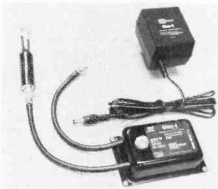
converter unit (mounted at the back of the TV set) and a 300 to 75 ohm transformer for the UHF terminals. All VHF channels 2 to 13, mid-band A to I and super-band channels J to R are converted to UHF channels 44 to 79.
