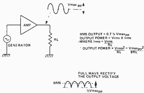
Therefore if  $RL=8R$  and  $V_{pp}$  is 1V,  $P_{(RMS)} = 15.6mW$ .
