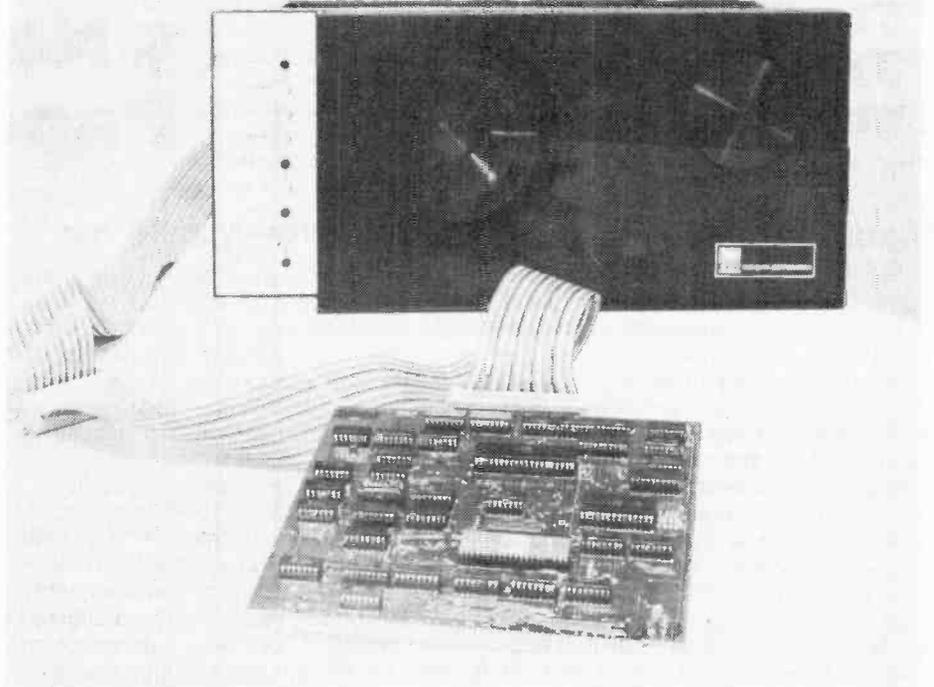
gaps and file marks. The tape decks are available in the three usual sizes with 7, 8½ or 10" reels. They operate on 115 or 230 VAC or, optionally, on 28 VDC.
