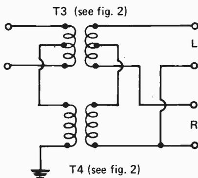
Fig. 5. Recovery of L and R signals in Simplex sum and difference system.
