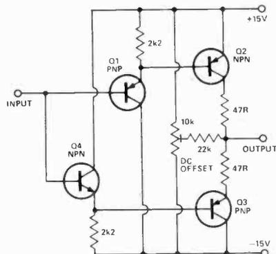
When you want to buffer a test generator to the outside world it is often very difficult to get an amplifier with sufficient bandwidth and power handling to do the job. The circuit is a very simple unity gain buffer. It has a fairly high input impedance, a 50 ohm output impedance, a wide bandwidth and high slew rate.
