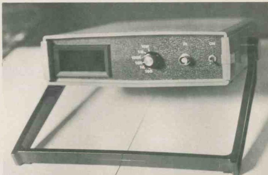
A FREQUENCY COUNTER is a very useful piece of test equipment as it can be used for troubleshooting both analog and digital circuitry. The design shown in this article uses readily available TTL and CMOS ICs for measuring frequencies from below 10 Hz up to 10 MHz.
