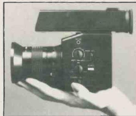
The Sanyo VSC800 is fairly new on the market. Like the RCA, it does not contain tape and must be used with a VCR, either Beta or VHS. Features include automatic focus and white balance, MOS image sensor, and a weight of just over one kilogram. One of its interesting features is a C-mount removable lens; this means that it will accept many 35 mm SLR camera lenses.
