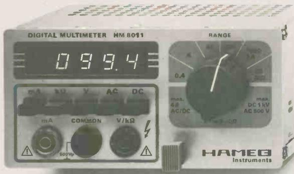
Apart from its **favourable price/performance ratio**, only on comparing features will be seen what this multimeter has to offer. Compared to most 3½ digit instruments with 2,000 counts, normally found in this price range, the **HM8011 features 4,000 counts**. This adds **one more digit of resolution** to all measured values in the top half of all ranges. In this way, the display corresponds to that of a 4½ digit multimeter with 20,000 counts.
