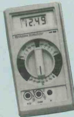
The HD-100 is built to be an indispensable tool in any environment. The tough fire-retardant case and the O-ring seals make the meter drop-proof and waterproof. The meter can withstand 600 volts without failure on all resistance ranges. Voltage ranges can withstand 6KV transients for 10 micro-seconds, and the 2 amp current ranges are protected by a 2A/600V fuse.
