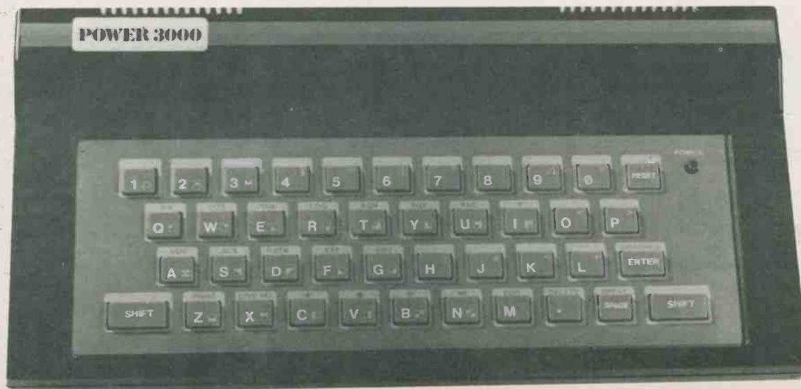
Yes, I did mention a speaker. As there is no true tactile feedback to the rubber keys, each keypress elicits a small 'bip' from the speaker to assure you that the struck key registered. After you pick up your typing speed, however, the audio feedback starts to sound like a bad rendition of *Popcorn*. Typing a quick 'NOBEEP' will silence the cacophony.
