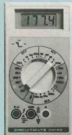
The DM40 is overload protected to 500 VDC/350 VAC in 0.2V range, and 1200 VDC/800 VAC in the other ranges.
