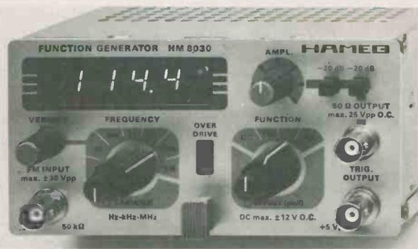
The various signals available from this module make the HM8030 a versatile signal source for most applications in test and measurement. The low frequency ranges are particularly well suited to simulate mechanical and servo techniques.
