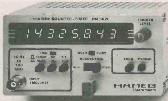
The capabilities of this counter/timer permit measurement of all frequencies from less than 1Hz up to 150MHz, as well as periods from 1 $\mu$ s to 100s. When operating the HM8020 as a system-unit, its input can be switched to provide rear panel interfacing capability between an oscilloscope and the mainframe unit HM8001.
