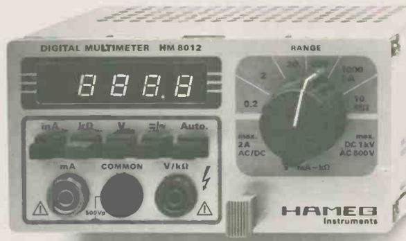
This digital multimeter measures voltage, current, and resistance with **increased accuracy and resolution** (4½ digits, 10 μV), featuring professional **autorange** convenience. Measurements are taken periodically at 0.4s intervals. **True RMS** capability provides more accurate AC measurements on distorted, noisy, random, or other nonsinusoidal waveforms. 100ms integration time effectively eliminate adverse influence from line power disturbances.
