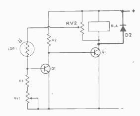
Fig. 10. A more controllable circuit with variable hysteresis.
