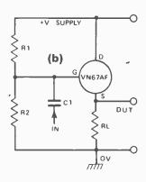
Fig. 12. Bias for common drain VMOS operation methods.
