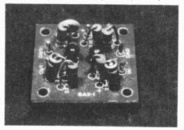
they are so sensitive, the circuit can switch to and fro when the conditions (light or temperature or whatever we are detecting) are steady around the changeover point. If the input is at the critical value at which the circuit switches, then the relay 'chatters' as the transistors switch on and then off again with each tiny fluctuation of light or temperature as the case may be.
