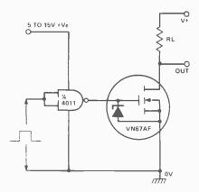
Fig. 7. Method of interfacing VMOS with CMOS!
