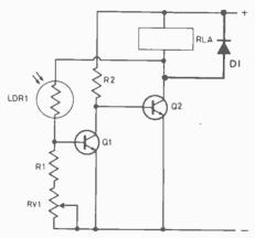
Fig. 9. A light-relay circuit with hysteresis (see text).
