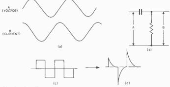
Fig. 2. The effects of capacitor coupling on low-frequency signals. (a) Phase shift of voltage relative to current, (b) in the coupling circuit, the output voltage (A) is not in phase with the input voltage (B) to the next stage. A low frequency square wave (c) becomes distorted to the spiked shape (d) unless very large capacitance values are used.
