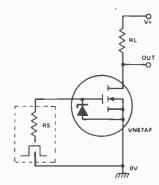
The rise and fall times of the output of the circuit are determined by the source impedance of the input signal, the input capacitance and forward transconductance of the VMOS device and the value of R<sub>L</sub>. If R<sub>L</sub> is large compared to R<sub>s</sub> the VN67AF gives rise and fall times of roughly 0.11 nS per ohm of R<sub>s</sub> resistance. Thus, a 100R source impedance gives an 11 nS rise or fall time.
