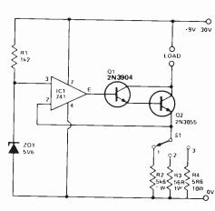
Q2 should be mounted on a suitable heatsink.
