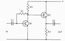
Fig. 5. Direct-coupling two stages together, using a shunt-feedback amplifier and an emitter-follower.
