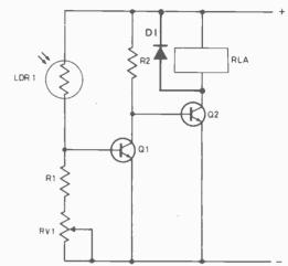
Fig. 8. More sensitive light-relay circuit.
