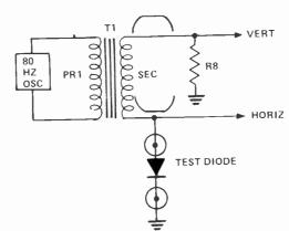
Fig. 5. Simplified diagram of the Huntron Tracker.
