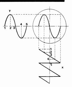
Fig. 1. Showing how the deflection waveforms applied to the X and Y plates of a cathode ray tube cause the electron beam spot to trace out a faithful replica of the Y-input waveform.
