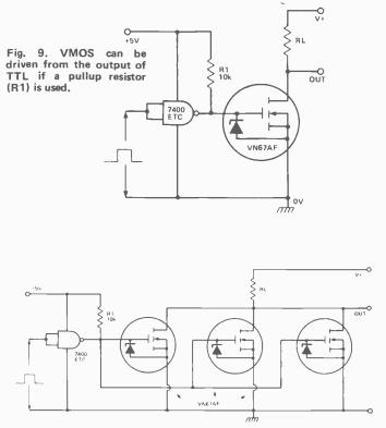
Fig. 10. Boosting the output of Fig. 9 by driving three VN67AF in parallel.
