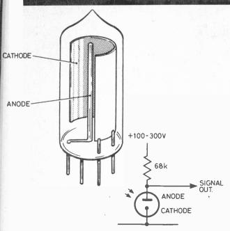
Fig. 2. A vacuum photocell, and typical circuit.
