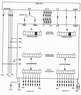
the direction register. After this the programmer will ensure that bit "2" is set to 1, so subsequent reference to 8004 will address the data register. It would be most unlikely to have to change the direction register contents in the same program, but if so, it would be necessary to clear bit "2" first and reset it again afterwards.
