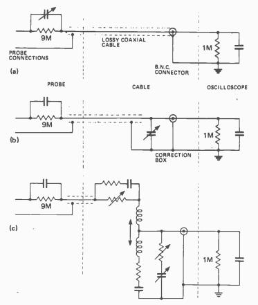
Fig. 4. Schematic of attenuator probes (a) simplest concept (b) capacitive loading to extend bandwidth (c) inductive.
