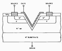
Fig. 2. Cross Section of a VMOS power FET.
