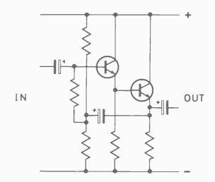
Fig. 12. A two-stage bootstrapped circuit with a very high input resistance of several megohms.
