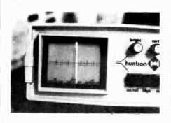
"LOW" range, transistor emitter to base, bad trace, leakage.
