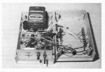
The case of Shark opened for inspection, using a large battery ensures the game will not suddenly die on you. Note C7 mounted next to the battery, using a PCB type makes the wiring easier.
