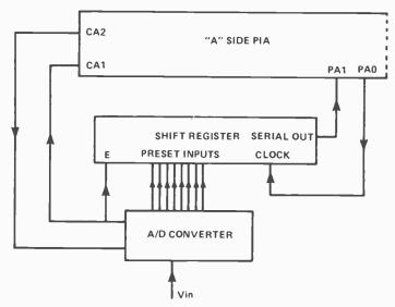
twenty wires if we insist on the minimum amount of extra hardware to convert. Suppose we are prepared to relax a little and allow a TTL shift register between the A/D and the PIA as shown in figure 5.
