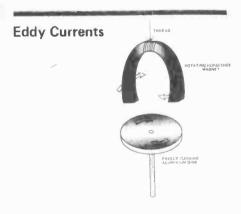
Eddy currents present peculiar problemsespecially in the design of transformers yet the heating effects produced by them are used in the manufacture of semiconductors. A.S. Lipson explains.
