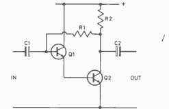
Fig. 4. Direct-coupling two stages together, using an emitter-follower and a common-emitter pair.
