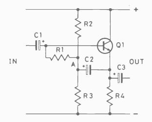
Fig. 11. A bootstrapped emitter-follower. The voltage at point A changes in phase with the input voltage, so that practically no signal cirrent flows through R1. The effect is similar to that of having a very large value of R1 for signals only.
