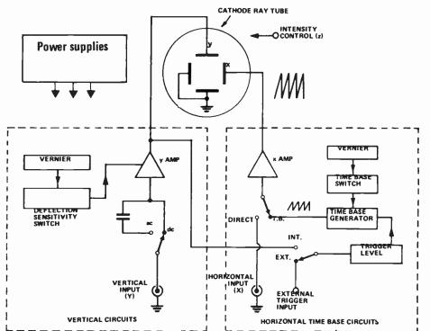
Fig. 2. Schematic diagram of essential sub-systems added to the CR tube to make it a measuring instrument.
