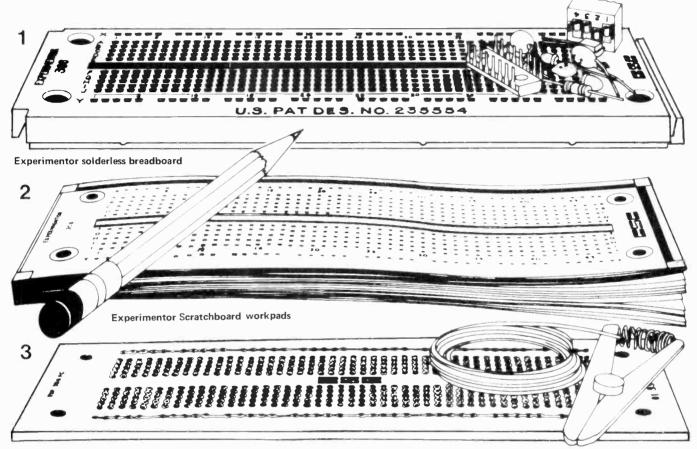
Experimentor Matchboard pre-drilled PCBs.
