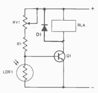
Fig. 7. Circuit for operating a relay when the light level drops.
