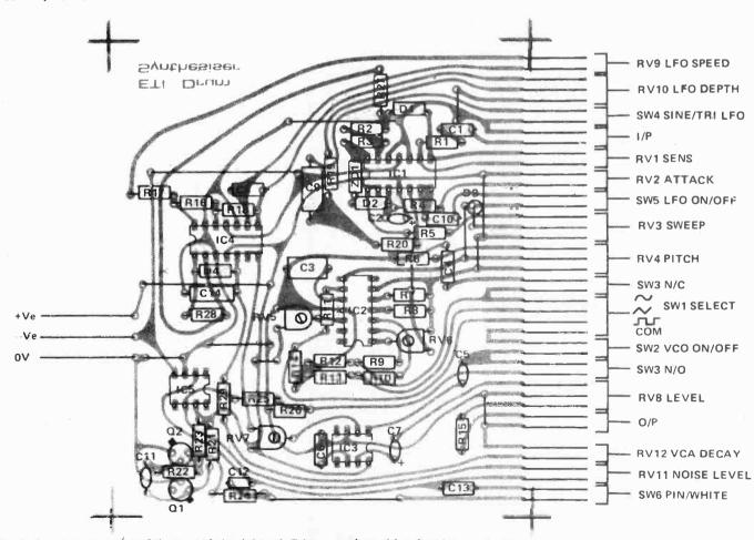
Fig. 7. Component overlay of the control circuit board. Take care when wiring the edge connector.
