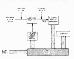
Block diagram logic state analyser.
