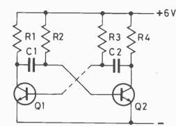
Fig. 13. The astable circuit. Try this out with the following values: R1, R4=3k3, R2, R3=33k, C1 C2=0.02 iF. Use an oscilloscope to examine the output waveform.
