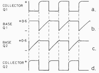
Fig. 14. Astable waveforms - these have been drawn to the same time-scale, with the vertical dotted lines linking changes which take place at the same time.
