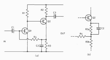
Fig. 6. A high gain two transistor circuit (a) with direct coupling negative feedback of signal can be achieved by removing C2, or by using the circuit in (b) where only part of R3 is bypassed.
