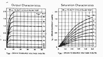
Fig. 3. Output and saturation characteristics of the VN67AF VMOS power FET.
