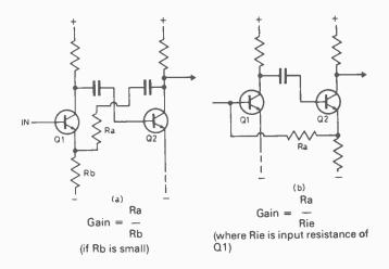
Fig. 3. Methods of connecting negative feedback over two stages. (a) Collector-to-emitter, (b) emitter-to-base.
