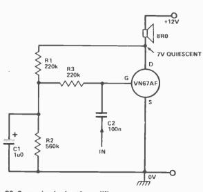
Fig. 20. Super simple class-A amplifier.
