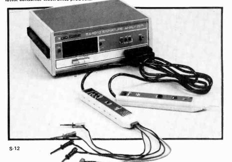
input, or address, function, the outputs will follow a logical course of events and give a final result dependant upon (a) the input function and (b) an internal clock function (if used). An instrument has been developed which injects a known digital signal (algorithm) into the inputs of the microprocessor. VCC, GROUND, STOP and START functions are provided as well as a CLOCK function.
