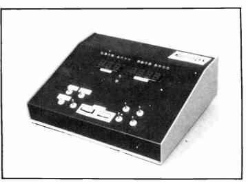
The Multiflex Logic State Analyzer allows a technician to quickly track down faults in the microprocessor system.
