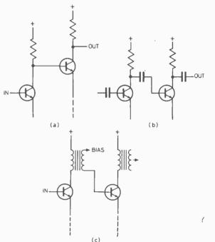
Fig. 1. Coupling methods (bias components omitted) (a) Direct (b) Capacitor, (c) Transformer.
