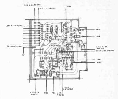
Fig. 2. PCB overlay for Shark. It's a good idea to use IC sockets.
