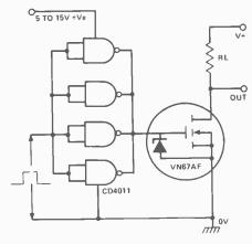
Fig. 8. VMOS switching times can be reduced by driving with a number of gates in parallel. Typical Rt = 25nS.
