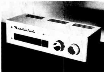
at each attenuator position. Output ranges (and therefore meter ranges) are 0-.003, .01, .03, .1, .3, 1, 3, 10 volts. Step-tuning provides rapid positive selection of the desired frequency, and allows accurate return to any given frequency.
