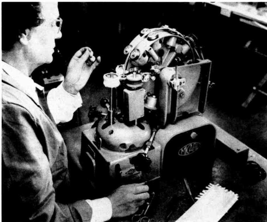
The Swiss-made MICAFIL RW-I Toroidal Coil Winding Machine in operation at Sperry Gyroscope Co. Ltd., Montreal, for precision winding of coils for the aircraft and electronics industry.
