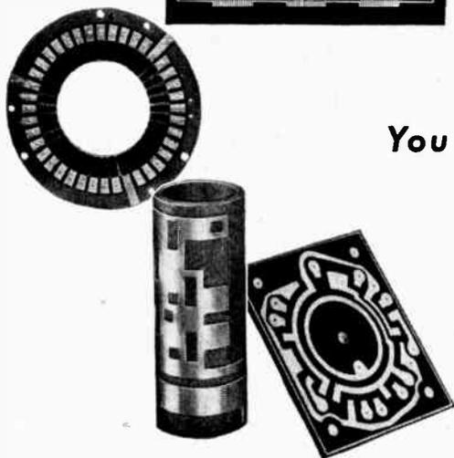
Switch plates, commutator discs, and drum commutators with printed circuits have proved themselves in many diversified applications. Low-cost printed circuit switches are ideal for simple switching, and show up to best economical advantage in complex switching functions.
