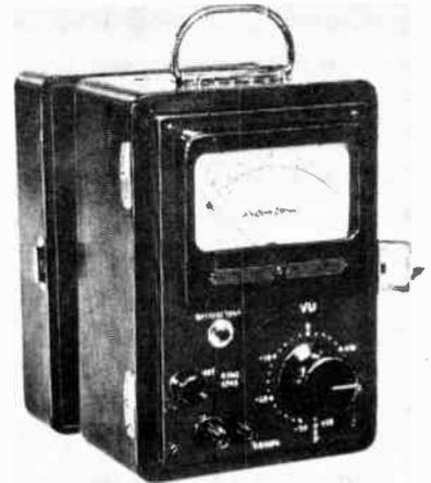
it through either binding posts or a telephone type jack and both bridging and terminating input impedances are available. Means are provided for checking the condition of the batteries and for adjusting the calibration.
