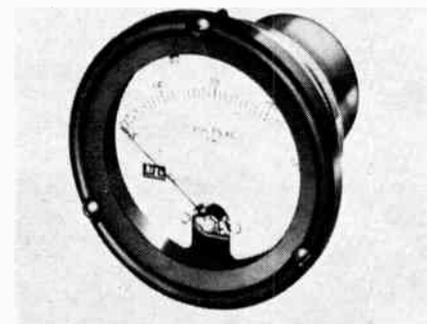
voltage which may be as low as 6.25 volts with a span of  $\pm 0.25$  volts, or as high as 230 volts with a span of  $\pm 30$  volts. A complete line of  $3\frac{1}{2}$ " and  $4\frac{1}{2}$ " diameter models is supplemented by square ( $3\frac{1}{2}$ "") and rectangular ( $4 \times 6$ "") models. Hermetically sealed and ruggedized models offer extreme durability under exacting conditions.
