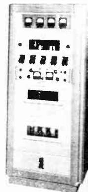
speed CW., radiotelephone, frequency shift keying, and facsimile transmission. A high level speech modulator is employed which provides clipping and limiting functions consistent with ample power.
