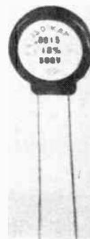
Iso-Kap is clearly labelled to avoid confusion and mistakes. Stamped with capacity, voltage rating, and tolerance.
