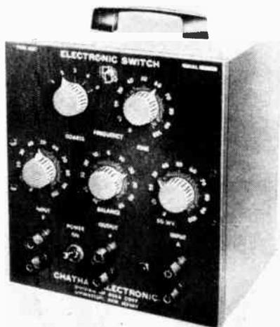
A square-wave voltage of variable frequency and amplitude is available at the output terminals for use as a test signal in studying the transmission characteristics of vacuum-tube amplifiers and other circuits.
