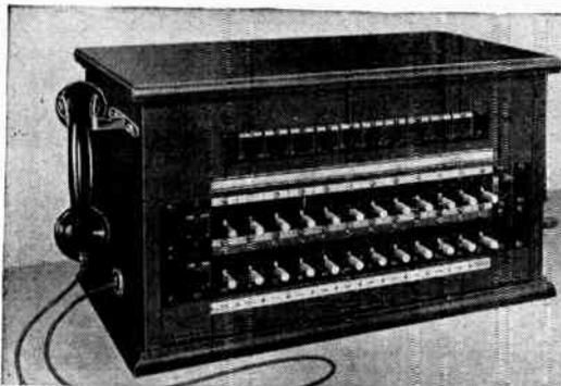
Cordless Switchboards, both C. B. and Magneto
