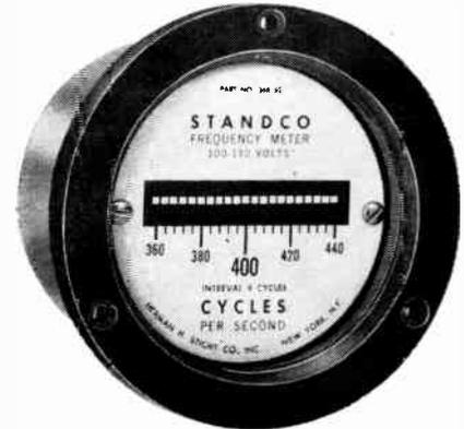
cycles, 50 cycles, 60 cycles, 400 cycles, 800 cycles and specials up to 1500 cycles; accuracy plus or minus 0.5 per cent. The individual reeds tuned to within plus or minus 0.3 per cent of their rated frequency; suitable for operation on 100-150 volts, 200-250 volts, 440 volts or low voltages. Trade name — "STANDCO", precision built, with reeds aged to prevent fatigue with resultant inaccuracies.
