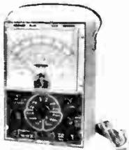
**ES-2**—The Stark ES-2, a 20,000 ohms volt circuit analyzer is a rugged compact instrument which offers accurate multi-range voltmeter, milliammeter and ohmmeter measurements over wide ranges.
