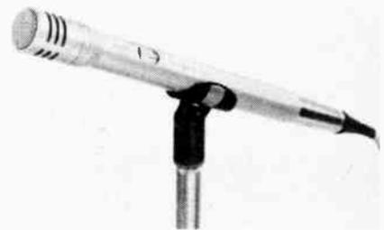
flat response, a rolloff of 6dB/octave below 100Hz or a cutoff of 18dB/octave below 80Hz. The mike includes a switchable 10dB attenuator built into the head to prevent overload to the internal electronics. It operates over a wide range of simplex powering voltages, and externally, its dimensions are a weight of 8 oz. and length of less than 8 1/2".
