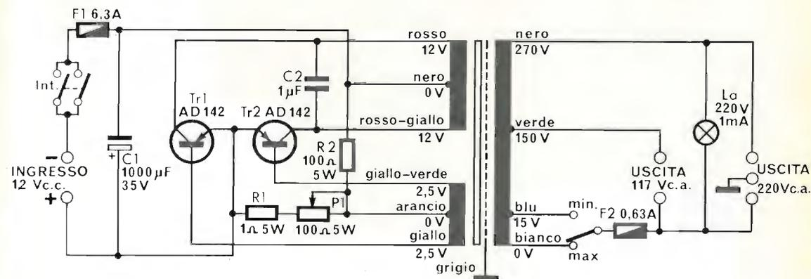
NB. LE TENSIONI SONO STATE RILEVATE A VUOTO A 50 Hz
