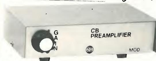
**P27-1 PREAMPLIFICATORE DI ANTENNA A MOSFET**
