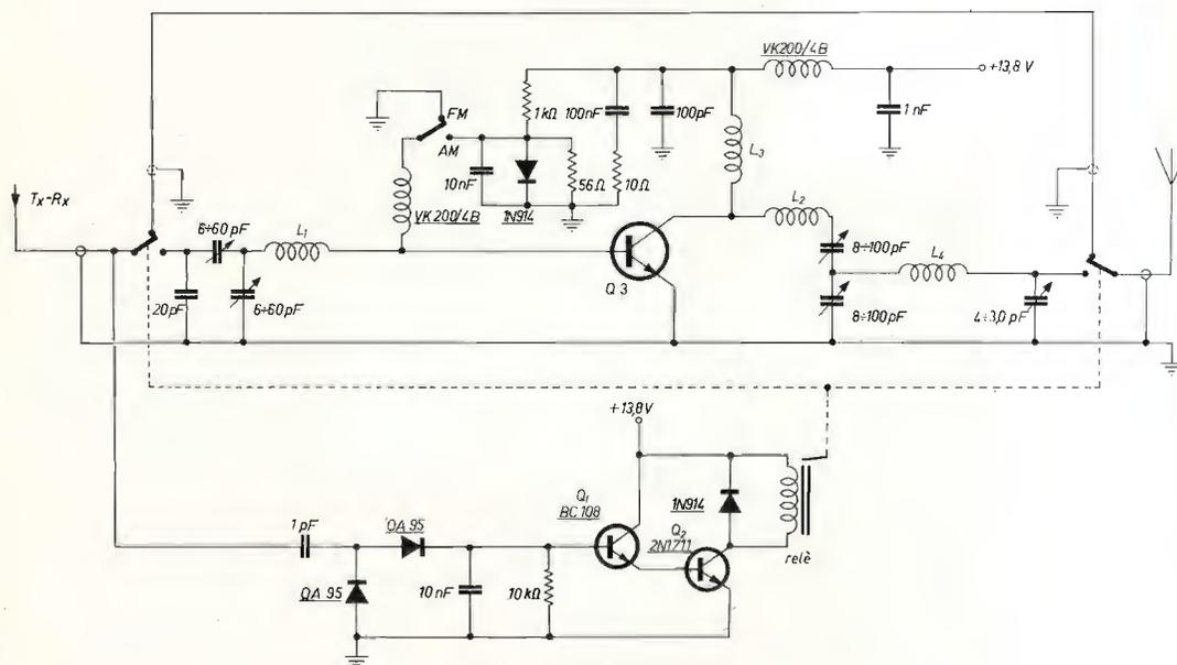
Transistor (Q<sub>3</sub>) B40-12 della CTC Communication (STE, Milano, via Maniago 15)
