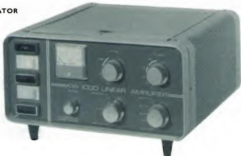
The K.W. 1000 Linear Amplifier is designed to be driven by the K.W. 2000A, or similar medium powered SSB Transmitters and Transceivers. Good linear operation is achieved for Single Sideband or CW with useful power gain.
