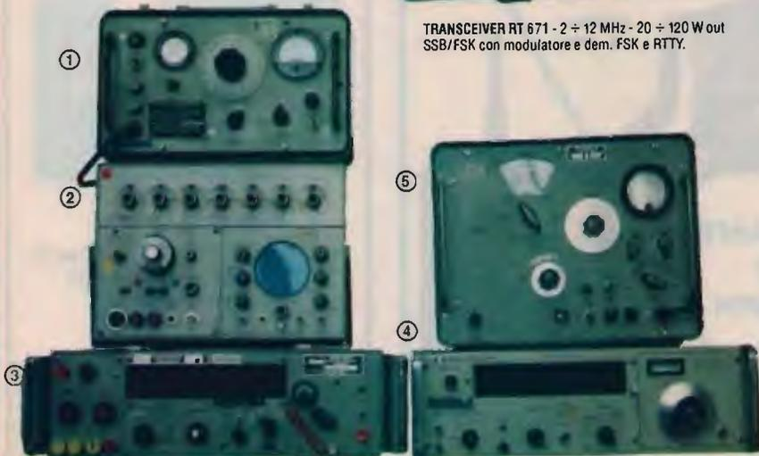
① Sig - gen. URM-127 - 0 ÷ 200 kHz, ATT+ALC • ② Test set AM/FM 0 ÷ 500 MHz • ③ Counter dig. read out CP-814A + CU1921A - Ris. 0,1 Hz/500 MHz • ④ Freqenzimetro HP5245L + 5253B - Ris. 0,1 Hz/500 MHz • ⑤ Sigm. Generator URM26 (-), 4-410 MHz, URM-25(-) 10 kHz-50 MHz.
