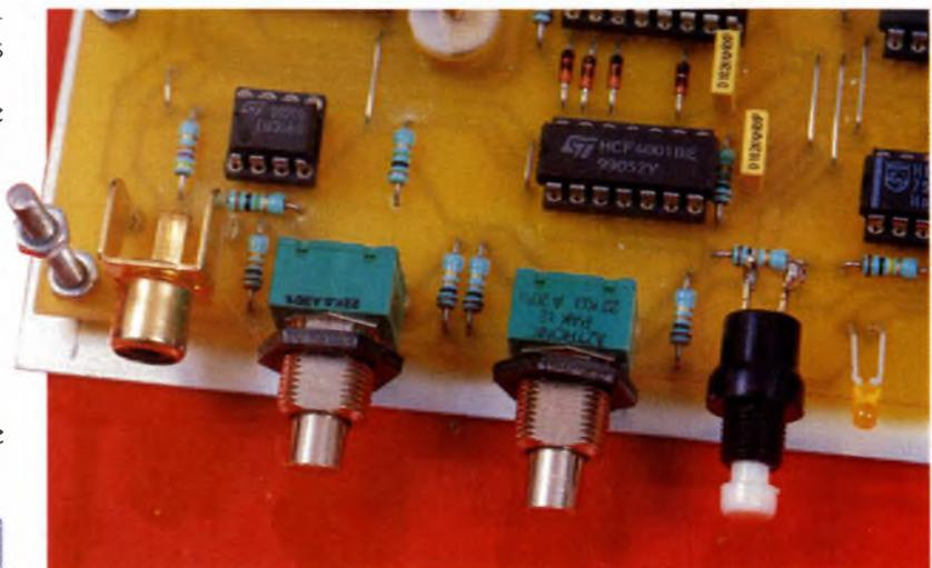
LES POTENTIOMÈTRES P<sub>1</sub> ET P<sub>2</sub>.
