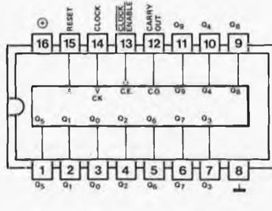
SYNCHRONOUS PRESETTABLE DIVIDE BY 'N' COUNTER
