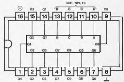
SYNCHRONOUS PRESETTABLE BINARY/DECADE UP/DOWN COUNTER
