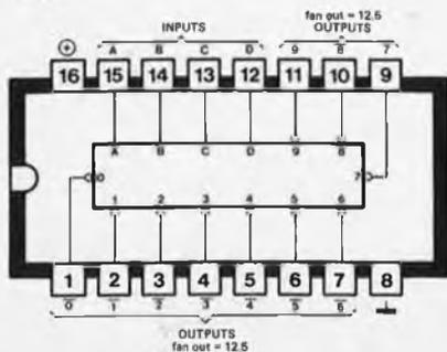
BCD TO 7 SEGMENT DECODER/DRIVER WITH OPEN COLLECTOR OUTPUTS
