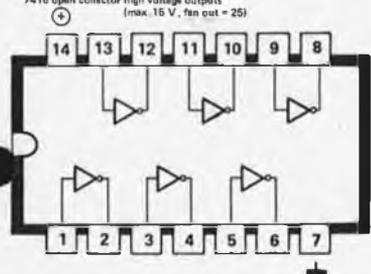
HEX BUFFER/DRIVER WITH OPEN-COLLECTOR HIGH VOLTAGE OUTPUTS (max. 30 V, fan out = 25)
