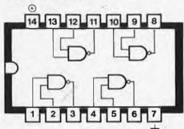
QUADRUPLE 2-INPUT NAND GATE WITH OPEN COLLECTOR OUTPUT
