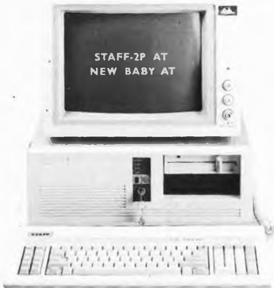
The model MS-21 uses new enhanced VLSI technology and high performance logic to run at either 8 Mhz or 10 Mhz clock speeds without wait states.
