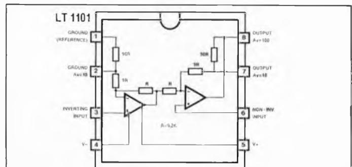
Ground pin 1, output at pin 8
