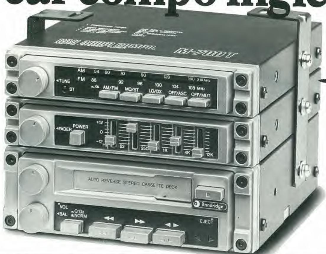
COMPLESSO STEREO HI-FI MODULARE COMPOSTO DI SINTONIZZATORE, AMPLIFICATORE/EQUALIZZATORE, RIPRODUTTORE CON AUTOREVERSE.
