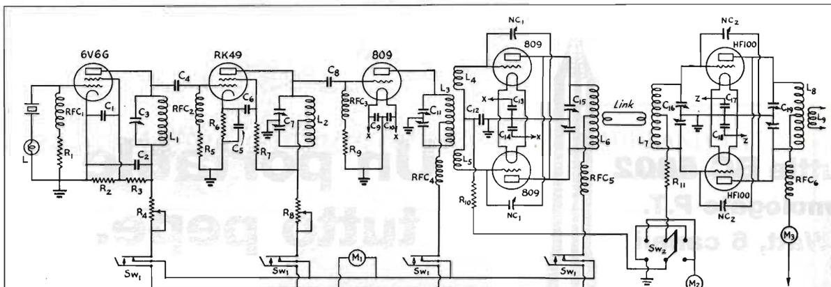
FIG. 1—CIRCUIT DIAGRAM OF THE COMPLETE R.F. SECTION
