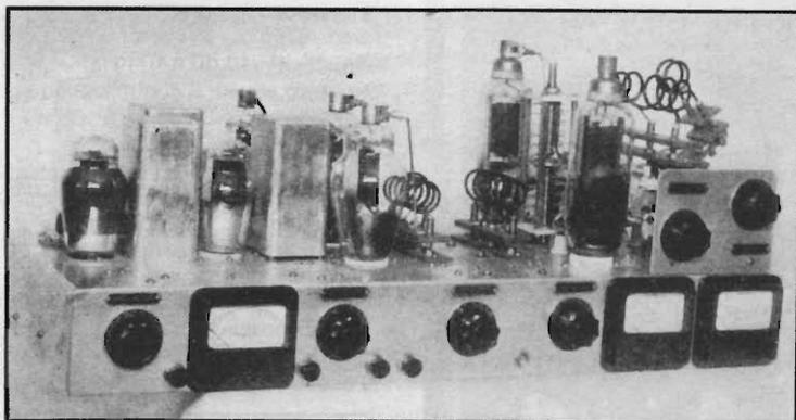
THIS 56- AND 28-MC. TRANSMITTER IS COMPLETE ON ONE CHASSIS
