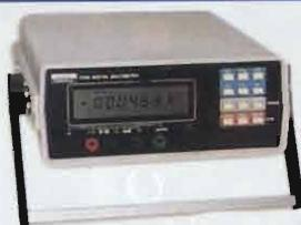
6 1/2 DIGIT - Misure: volt, test diodi,
