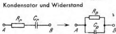
$$R_p = \frac{1 + (\omega C_r R_r)^2}{\omega^2 C_r^2 R_r}; \quad C_p = \frac{C_r}{1 + (\omega C_r R_r)^2}; \quad \text{tg } \varphi_p = -\frac{1}{R_r \omega C_r}$$
