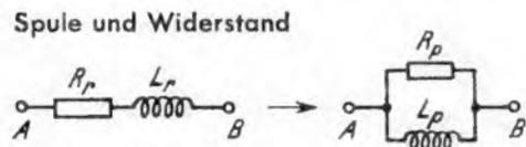
$$R_p = \frac{R_r^2 + (\omega L_r)^2}{R_r}; \quad L_p = \frac{R_r^2 + (\omega L_r)^2}{\omega^2 L_r}; \quad \text{tg } \varphi_p = \frac{\omega L_r}{R_r}$$
