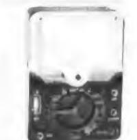
**M 200/TE 58** 20.000 Q/V V=0,6/30/120/600/1200 V = 6/30/120/600/1200 V A=0,06/6/60/600 mA  $\Omega$  10 100 K $\Omega$ /1 M $\Omega$ /10 M $\Omega$  C 0,007 - 0,2  $\mu$ F dB = -20 bis +63 Output-Messung **56,90**
