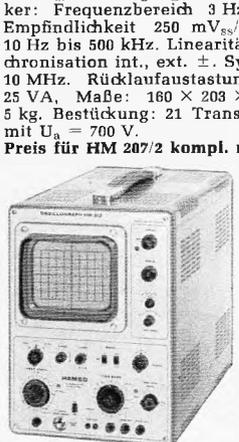
**TRIGGER-Oszillograph HM 312/3**
