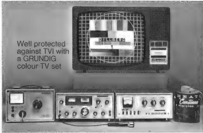
Test place with amateur transmitter and linear final stage for the control of television interference (TVI) at Grundig Super Color colour TV sets (see Funkschau number 24/1974)
