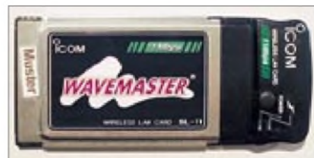
Wireless LAN à la Icom: Der 2,4-GHz-Transceiver SL-11 verbindet drahtlos PCs.
