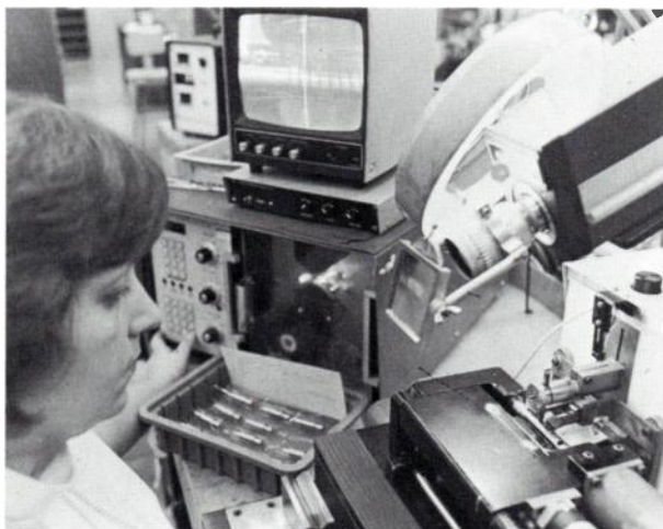
Fig. 19. — Automated disk-wire welding station.
