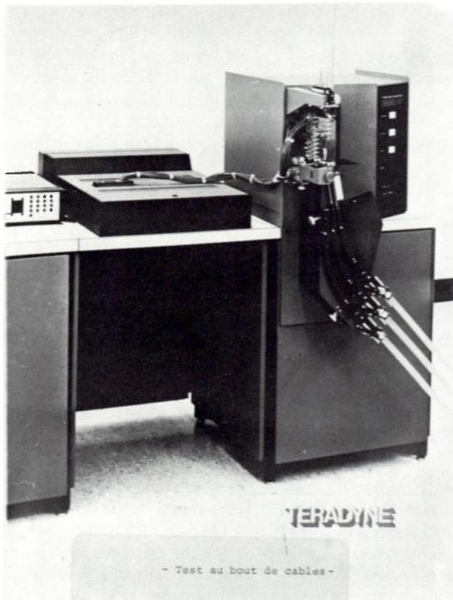
Fig. 7. — The J387 can test dynamically at the end of cables, this permits stringent testing at wafer probe and the use of mechanical handlers for the packaged circuit.
