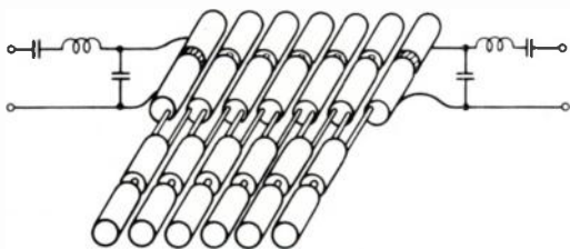
Fig. 20. — Channel EM filter with necked resonators (Kokusai Electric Co.).
