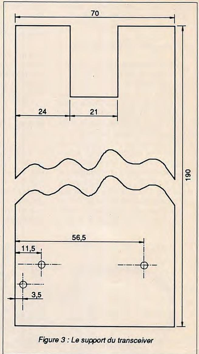
Figure 3 : Le support du transceiver
