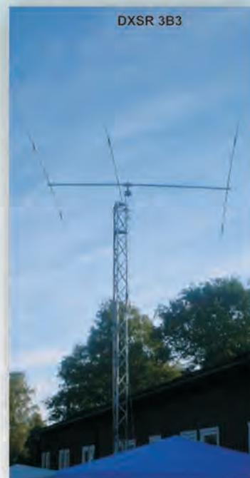
**2B3:** Yagi 2 éléments 10/15/20 m, 2 000 W, Gain 4.1 dBd (6.2 dBi), Av/Ar - 11 dB, boom 2.50 M
