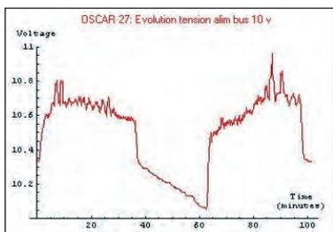
Figure 2: AO27 tension alimentation bus 10 V.
