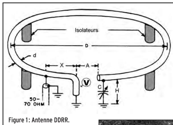
Figure 1: Antenne DDRR.
