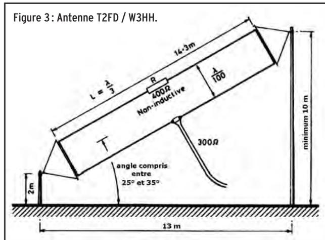
Figure 3: Antenne T2FD / W3HH.
