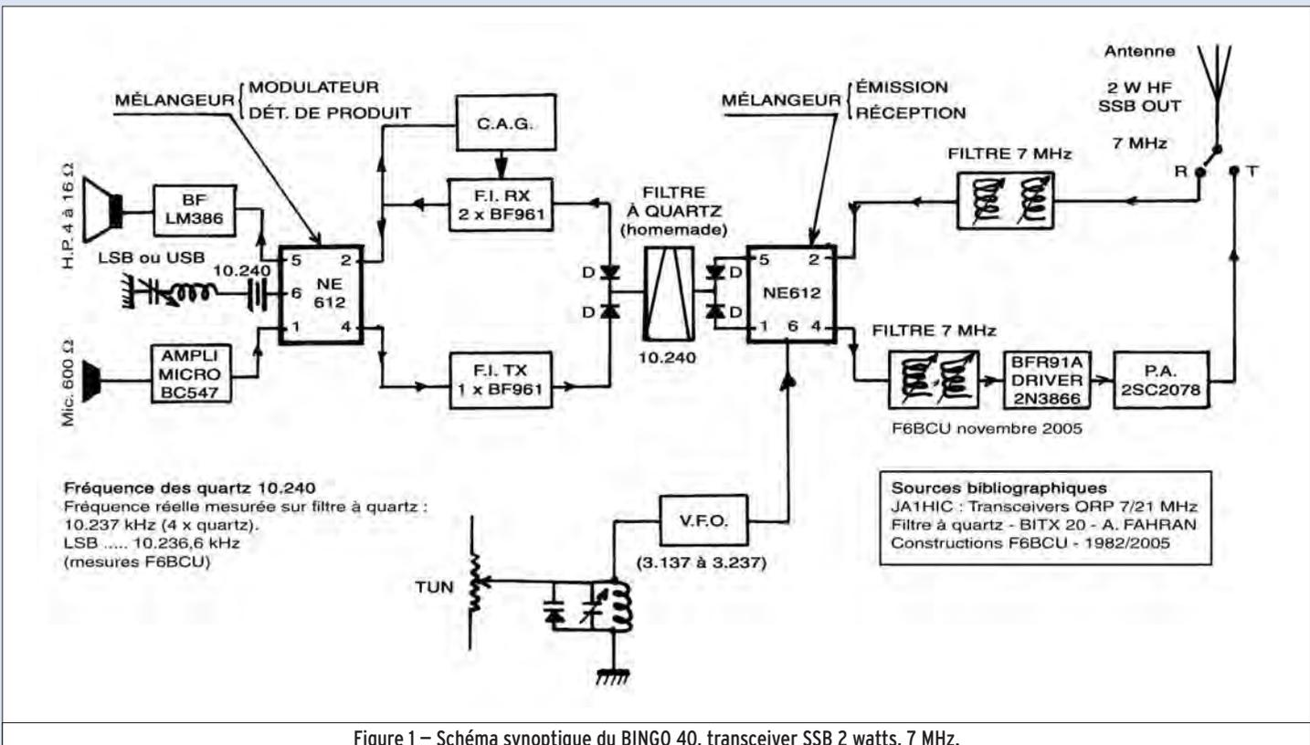
Figure 1 – Schéma synoptique du BINGO 40, transceiver SSB 2 watts, 7 MHz.
