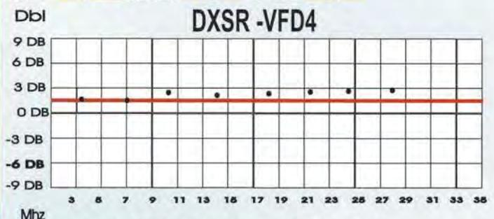
GAIN EN REFERENCE DIPOLE FULL SIZE DIPOLE = 2.15 dbi
