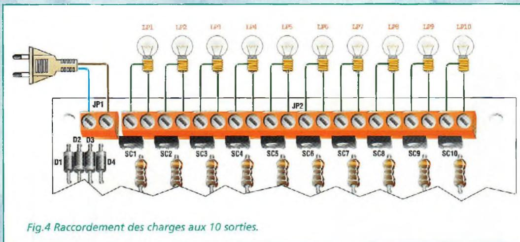
Fig.4 Raccordement des charges aux 10 sorties.
