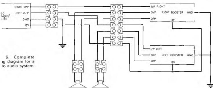
6. Complete wiring diagram for a stereo audio system.
