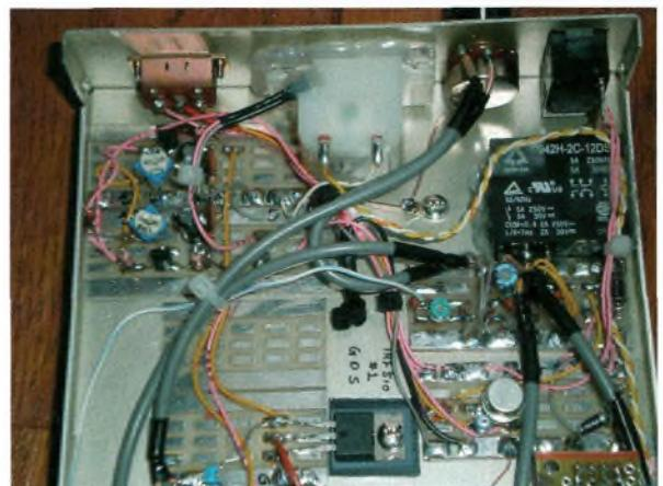
Experimental Only ! - QRP Booster using IRF-510 x 2 Pushpull Class-AB Linear Amplifier <Rev.0>
