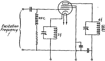
FIG. 1—THE FUNDAMENTAL CIRCUIT OF THE "DOUBLE-DOUBLER"
