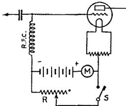
FIG. 4—BY CHOICE OF SUITABLE RESISTANCE VALUE AT R, THIS CIRCUIT WILL ELIMINATE BIAS FLUCTUATIONS AND PREVENT DAMAGE TO BIAS BATTERIES CAUSED BY GRID-CURRENT FLOW
