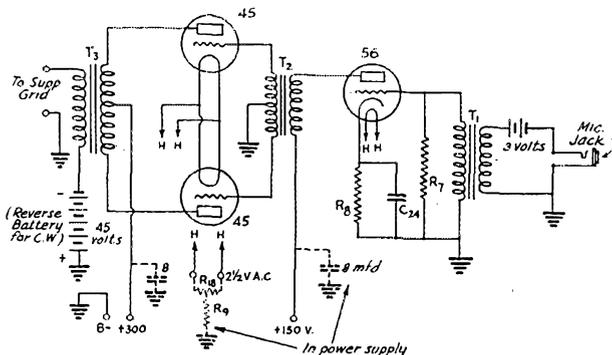
FIG. 3—THE SINGLE-STAGE SPEECH AMPLIFIER AND MODULATOR CIRCUIT
