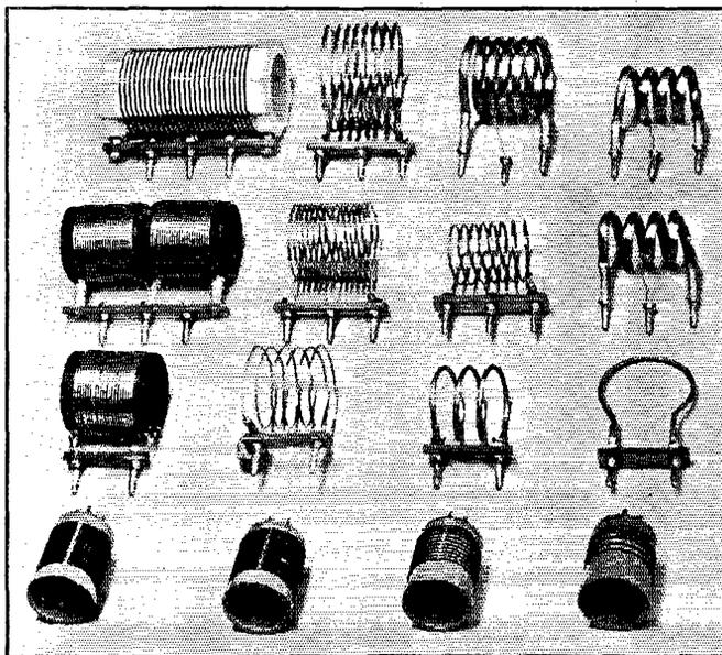
ILLUSTRATING THE FIVE TYPES OF COIL CONSTRUCTION USED
