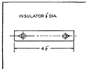
**ANTENNA INSULATOR.** This insulator is particularly suited for general use by the amateur. Its length provides ample leakage path, while its cross-section provides ample strength for all but the heaviest loads. The use of Steatite assures excellent electrical performance.
