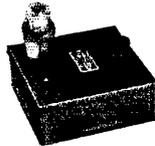
A type 30 tube is used, and four flashlight cells in the case provide the necessary filament and plate current.
