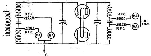
FIG. 7 — CIRCUIT FOR MEASURING PLATE AND GRID CURRENTS OF INDIVIDUAL TUBES IN A PUSH-PULL AMPLIFIER
