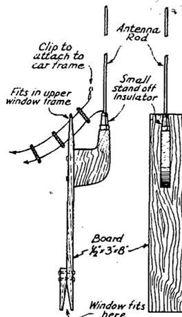
FIG. 2 — DEMOUNTABLE FIVE-METER ANTENNA FOR THE CAR
