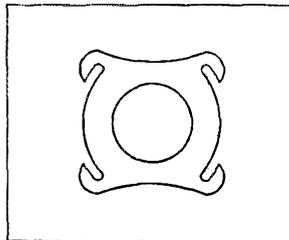
**TRANSPOSITION BLOCK.** In addition to the popular AA-1 Victron Block, National now offers a smaller Steatite Block. Both are light in weight, both are highly efficient. The Victron Block AA-1 separates feeders 1 1/2", the Steatite Block, AA-2, provides 1" separation.
