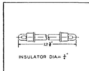
**ANTENNA INSULATOR.** Designed for sustaining heavy loads, this insulator combines great strength with low losses. The Steatite bar is  $\frac{3}{4}$ " diameter and has a leakage path of  $8\frac{1}{4}$ ". The fittings are of bronze. The weight of the complete insulator is approximately one pound.
