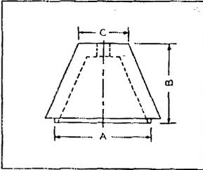
**H.F. BUSHING.** This small Steatite bushing has a variety of uses in transmitter construction, not only as a neat and efficient means of bringing H.F. leads through partitions, but as a support for coils, etc. Each pair of cones includes suitable metal fittings.
